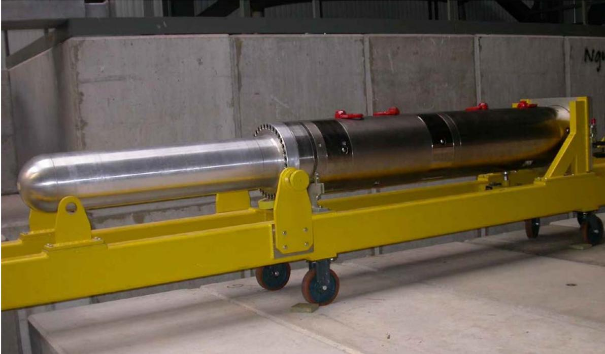
*Figure 2: Neutron spallation target, ready for installation and operation.*
