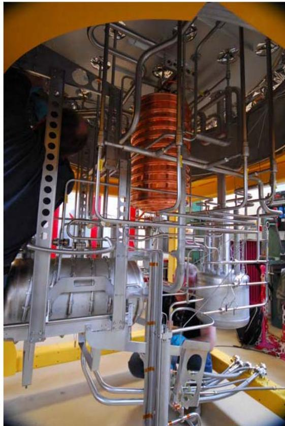
Figure 10: Heat exchanger components. 1: upper part of vacuum box, 2: condensation vessel for freezing the deuterium, 3: para-to-ortho deuterium converter.
