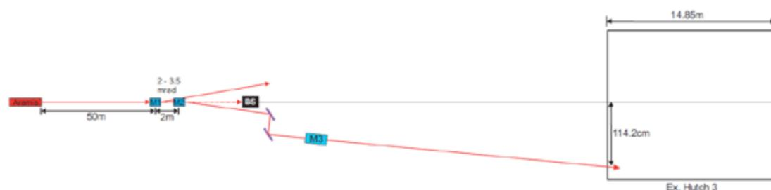
Fig. 4.3.2.4: Optics layout of the experimental hut 3. The beam separation distances shown are valid for a grazing angle of 3.5 mrad ( $0.2^\circ$ ).
