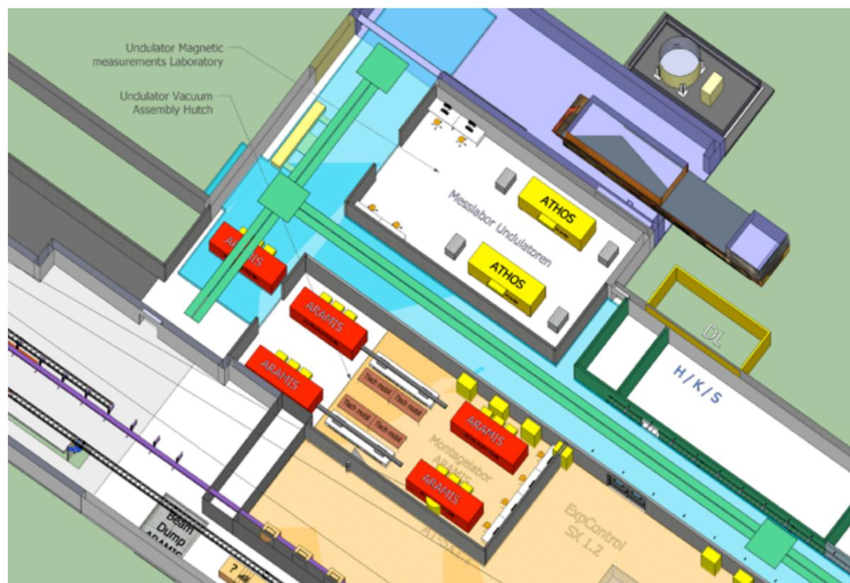
Fig. 5.3.1.1: Undulator Magnetic measurements lab and assembly hutch.
