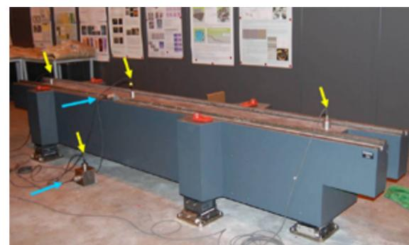
Fig. 3.8.4: Girder during eigenfrequency measurements: the arrows indicate the location of the accelerometers; test location at the SLS facility.
