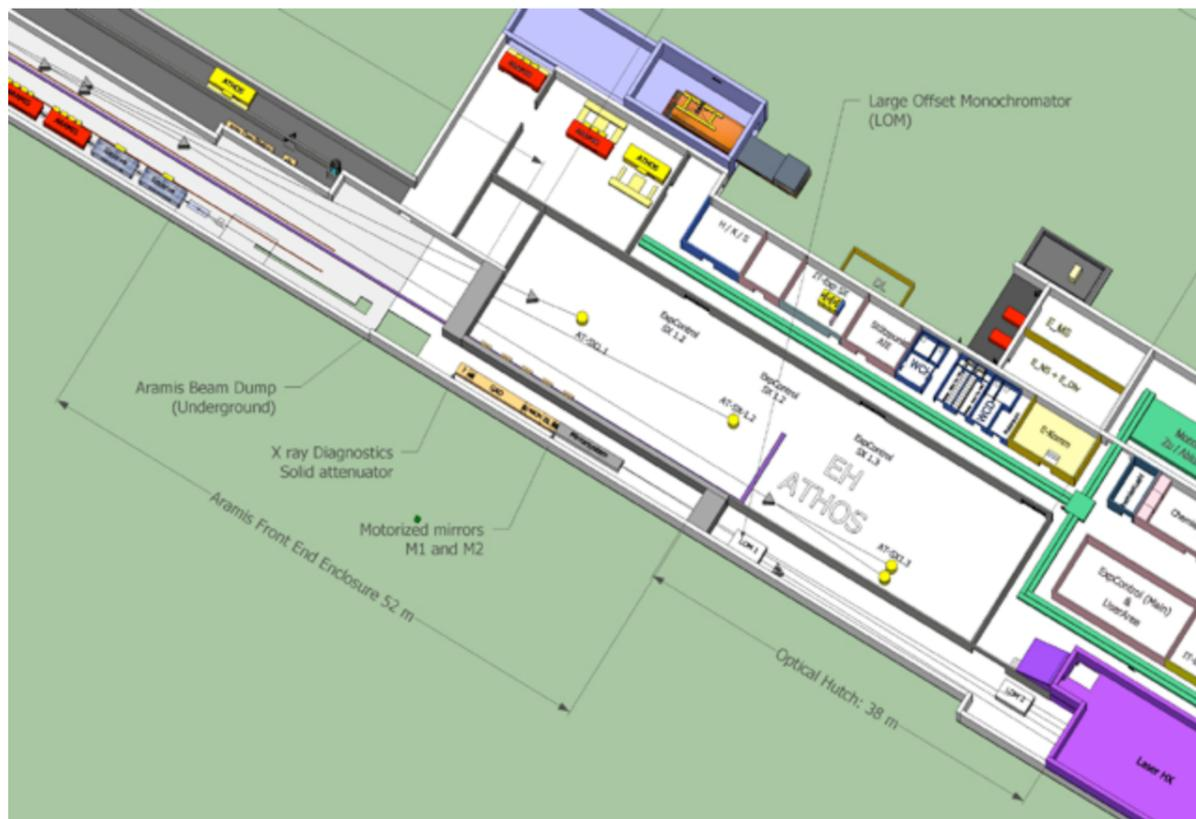
Fig 4.1.2: Layout of the Aramis Front End section and Photon Switch Yard section, behind the shielding wall.
