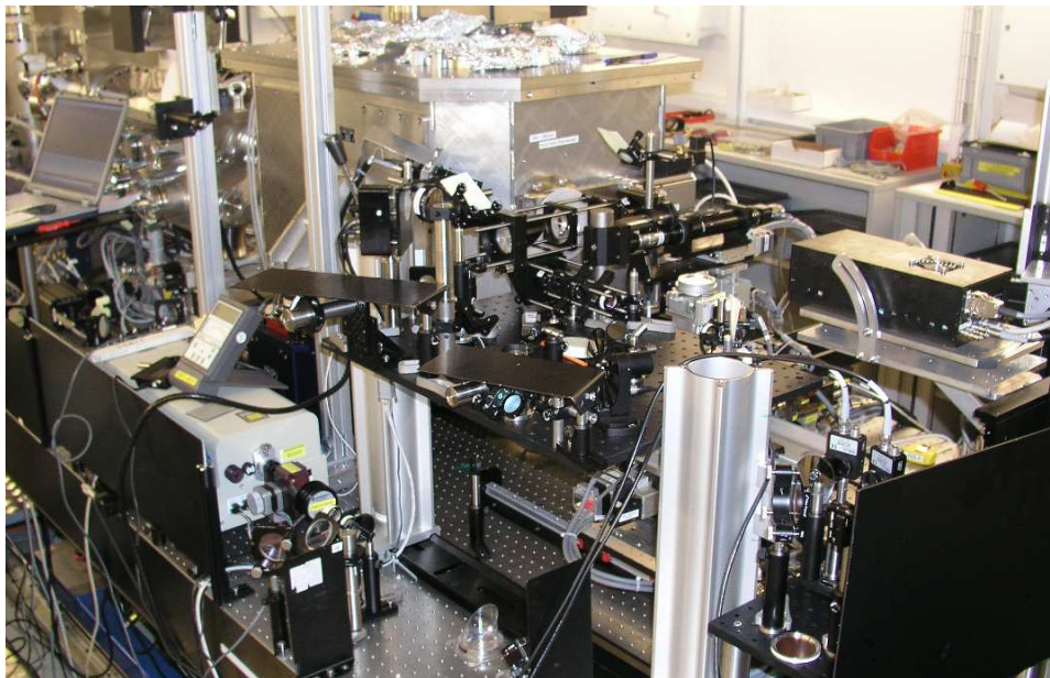
Figure A.1: Present R&D work relevant for the ARAMIS ES-B instrument: XPP vacuum chamber and THz-pumping.
