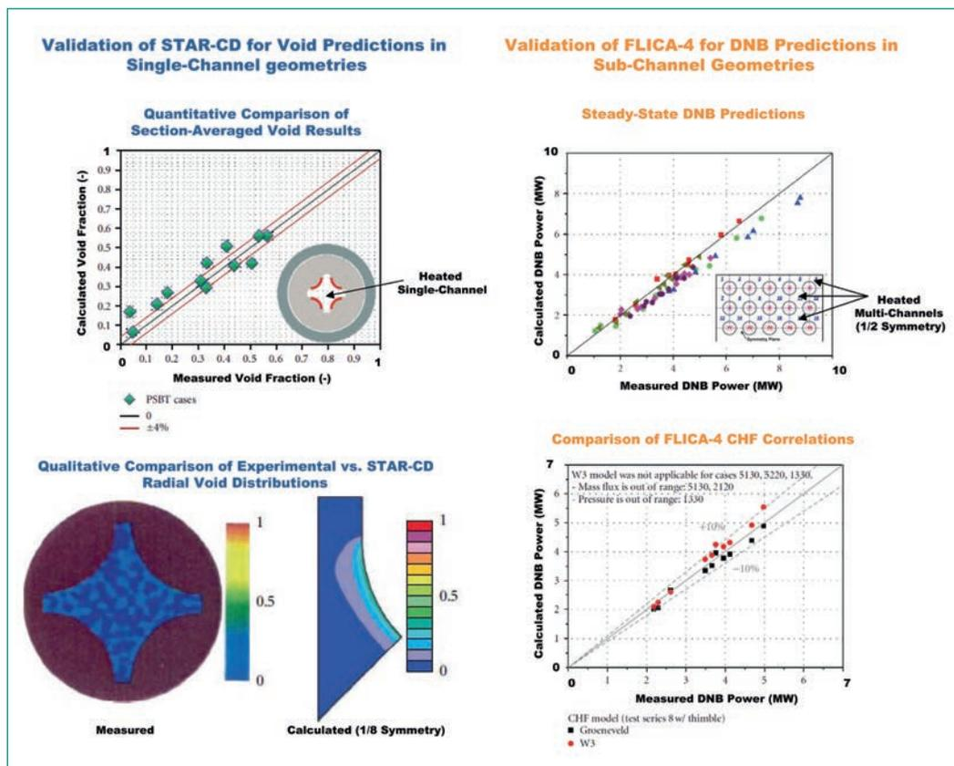
Figure 5: Modeling and Analysis of OECD/NEA PWR PSBT Void and DNB Benchmark with CFD (STAR-CD) and Sub-Channel (FLICA-4) Codes
