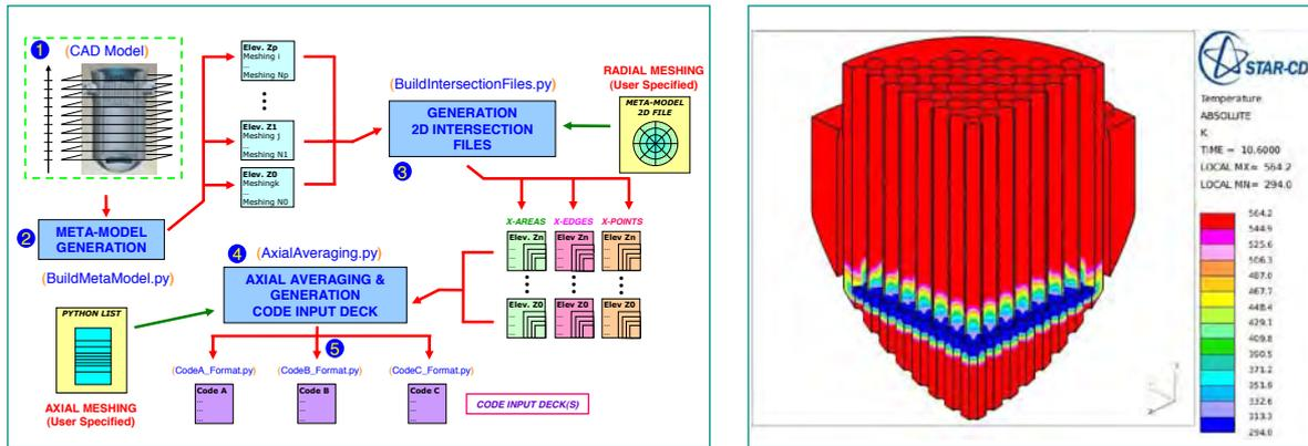
Figure 5: Architecture of a 3-D coarse mesh pre-processing tool for plant system codes (Left) and temperature distribution in KKL lower plenum computed by means of CFD (Right).
