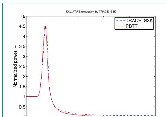
Figure 4: PB2 TTRIP Benchmark Relative Core Power.
