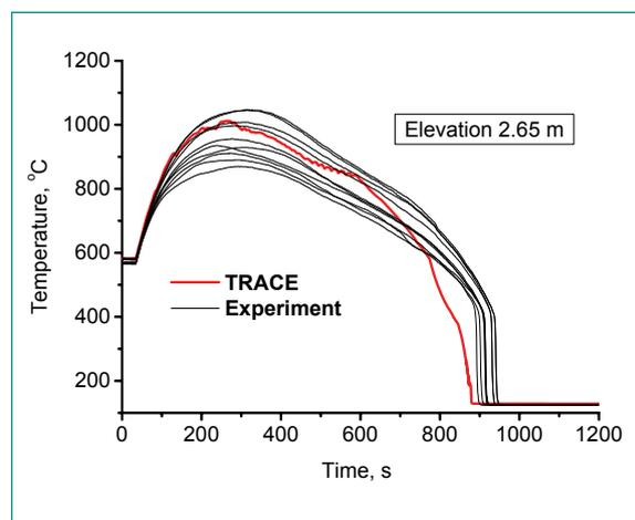
Fig. 13: Cladding temperature during reflooding (RUN A1R029).
