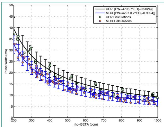
Fig. 17: PWR REA Pulse width Curves for UO<sub>2</sub> and MOX cores – CORETRAN/S3K Analyses.
