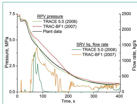
Fig. 7: Reactor pressure and liquid flow through SRVs.
