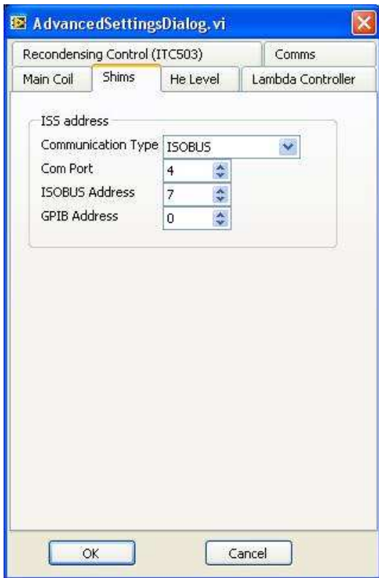
The Shims settings page. This page is used to configure the communications to the ISS10.
