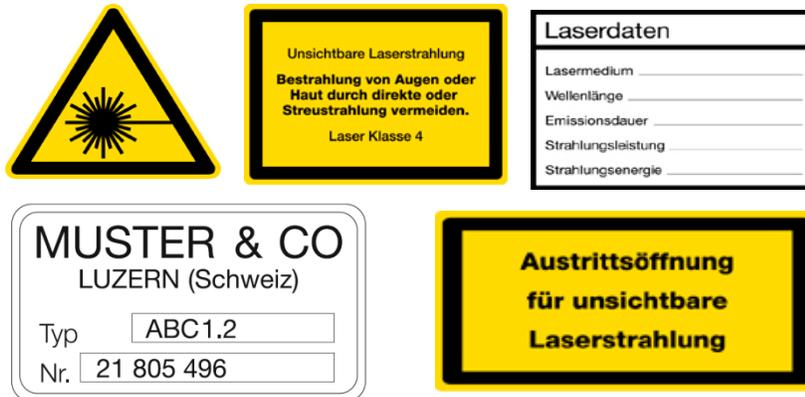
Figure 1: Laser labeling plates
