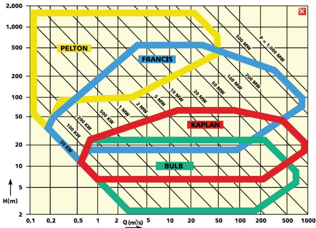
Figure 6.6: Application of different turbine technologies, depending on useable water head and flow rate.<sup>130</sup>
