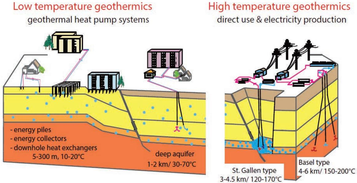
Technologies can be categorized based on the way thermal energy resources are used:
