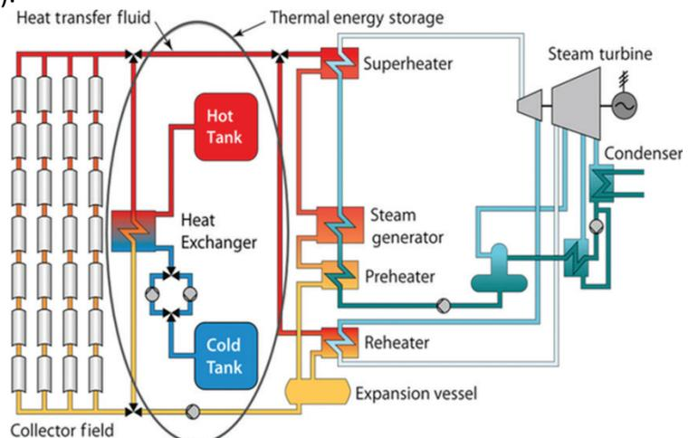
**Figure 13.10: Parabolic through plant with two tank indirect heat storage (Siegel 2012).**
