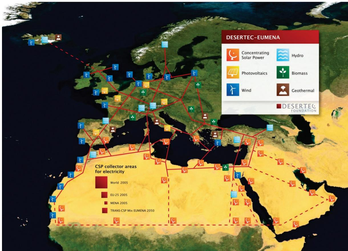
Figure 13.3: Vision of a European Mediterranean electricity grid based on HVDC lines for the use of the most efficient renewable energy resources, such as CSP, biomass, hydro, geothermal, wind, and solar PV. Indicated are possible power lines and future grid expansion. Also shown is the CSP collector area needed to cover the annual electricity demand of various world regions. Source: the DESERTEC foundation<sup>339</sup>.
