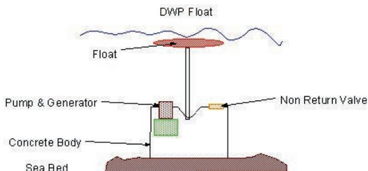
**Figure 12.10: Schematic Diagram of Seabed Piston Pump Design.**<sup>306</sup>
