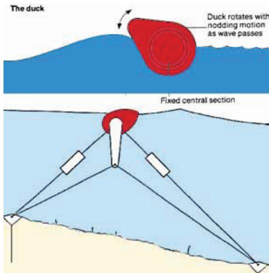
Figure 12.7: Schematic Diagram of Salter Duck Design.<sup>302</sup>
