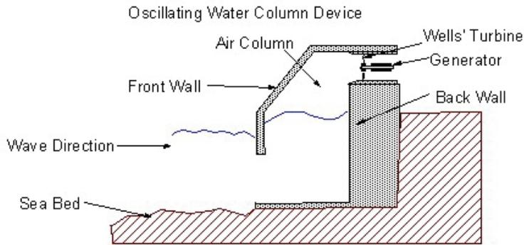
**Figure 12.3: Schematic Drawing of Oscillating Water Column Design.**<sup>298</sup>
