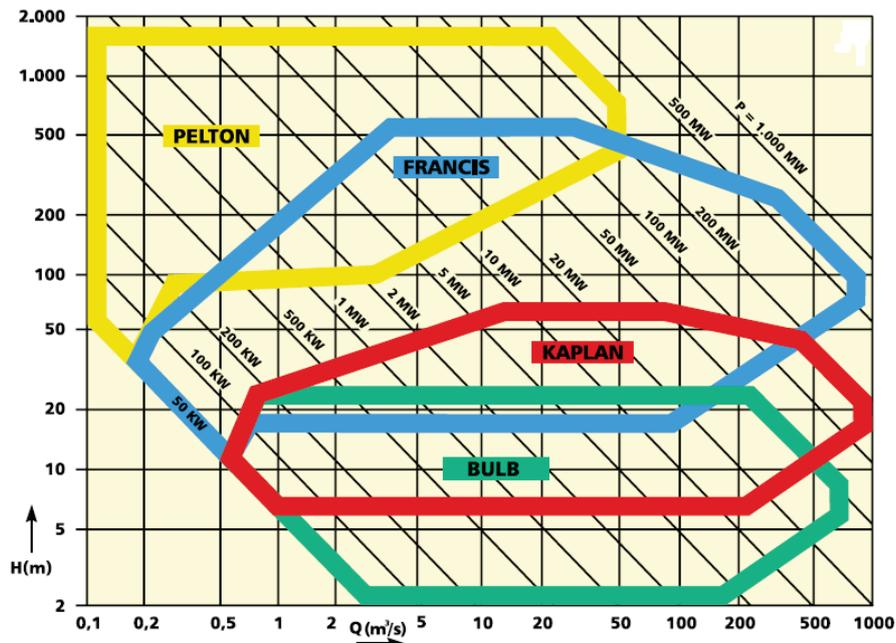
Figure 7.4: Optimal efficiency regime, as a function of flow rate and head, for different turbine types.<sup>140</sup>
