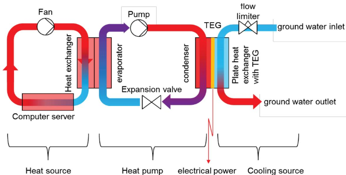
Figure 17.18: Scheme of a simplified cooling cycle for a heat source, e.g. a server room, with thermoelectric generators (Battaglia, Widmer et al. 2016).
