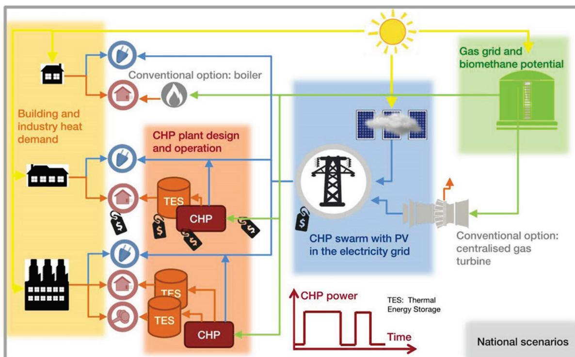
Figure 10.47: Operational strategy of the biomass swarm. Centralised swarm controller, local storage of heat and balancing the electrical grid on demand (Vögelin, Georges et al. 2016).
