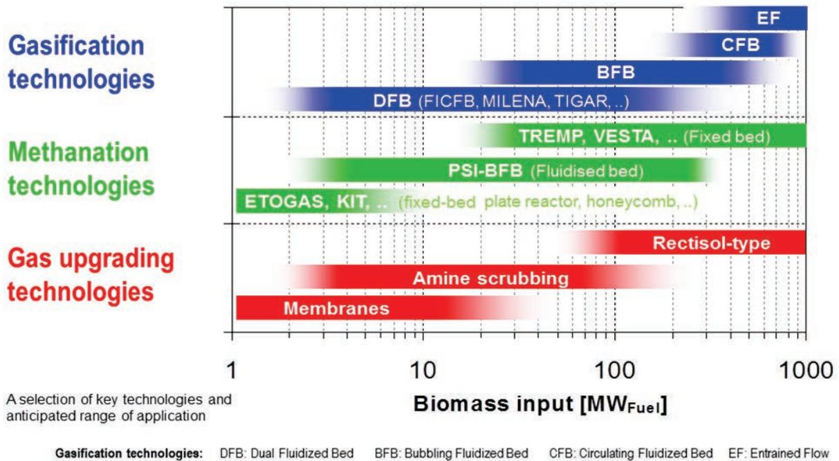
Figure 10.3: A selection of key technologies for biomethane production from woody biomass (Biollaz, Schildhauer et al. 2015).
