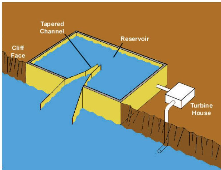
Figure 12.6: Schematic Drawing of Tapered Channel Design.<sup>301</sup>
