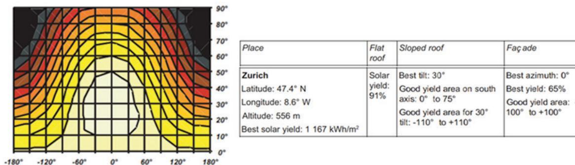
Figure 9.24: Annual solar yield for roof and façade PV installations in Zurich (IEA 2002).
