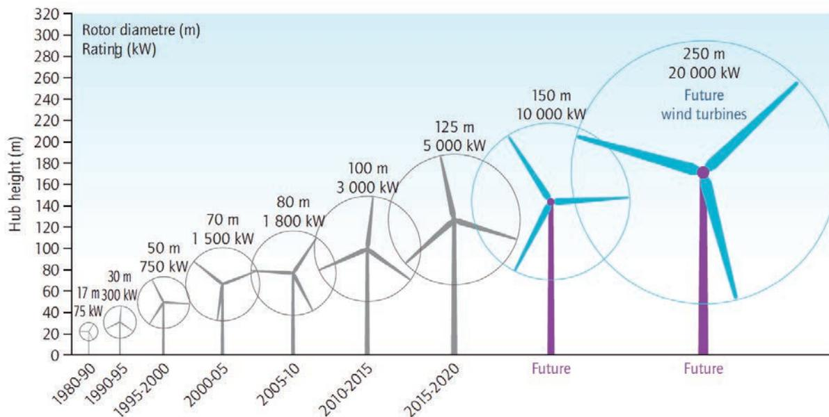
**Figure 8.19: Evolution of hub height, rotor diameter and rating of wind turbines over time. Taken from (IEA 2013a)**
