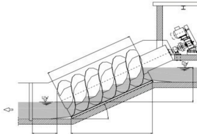
Figure 7.5: Concept of Archimedes screw turbine. Source: (BFE/SFOE 2011).
