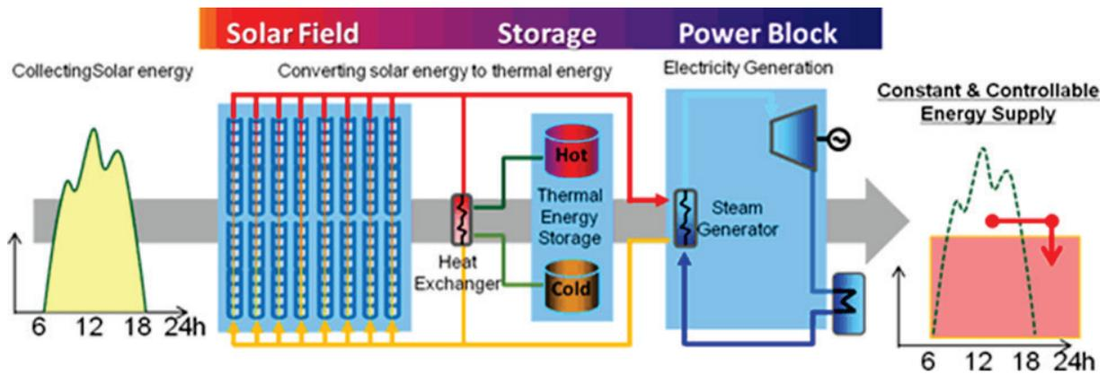
Figure 13.4: Schematic of a CSP system consisting of solar field, storage system and power block (Chiyoda 2016).
