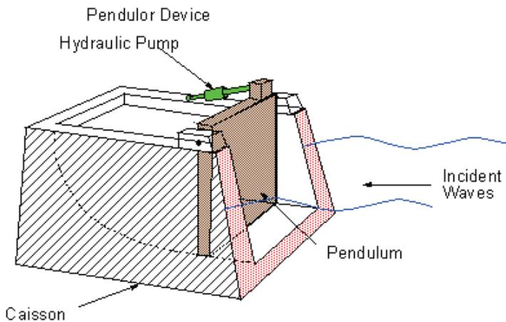
Figure 12.5: Schematic Drawing of Pendulum Design.<sup>300</sup>
