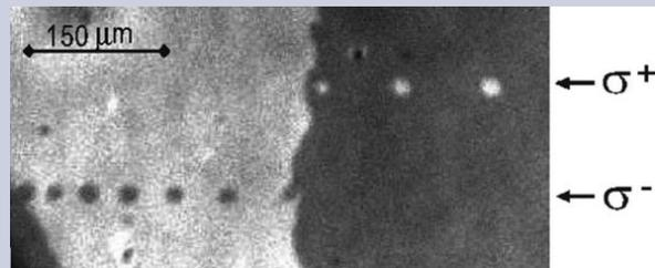
Fig. I.i5. Magnetic microstructures written into GdFeCo with right- and left- circularly polarized light [17]. The ATHOS beam-line at SwissFEL will allow the investigation of this process on fs and nm scales, which is important both for a microscopic understanding and for potential data storage applications.
