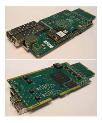
Figure 6: Pictures of the top and bottom side of the JUNGFRAU readout PCB.
