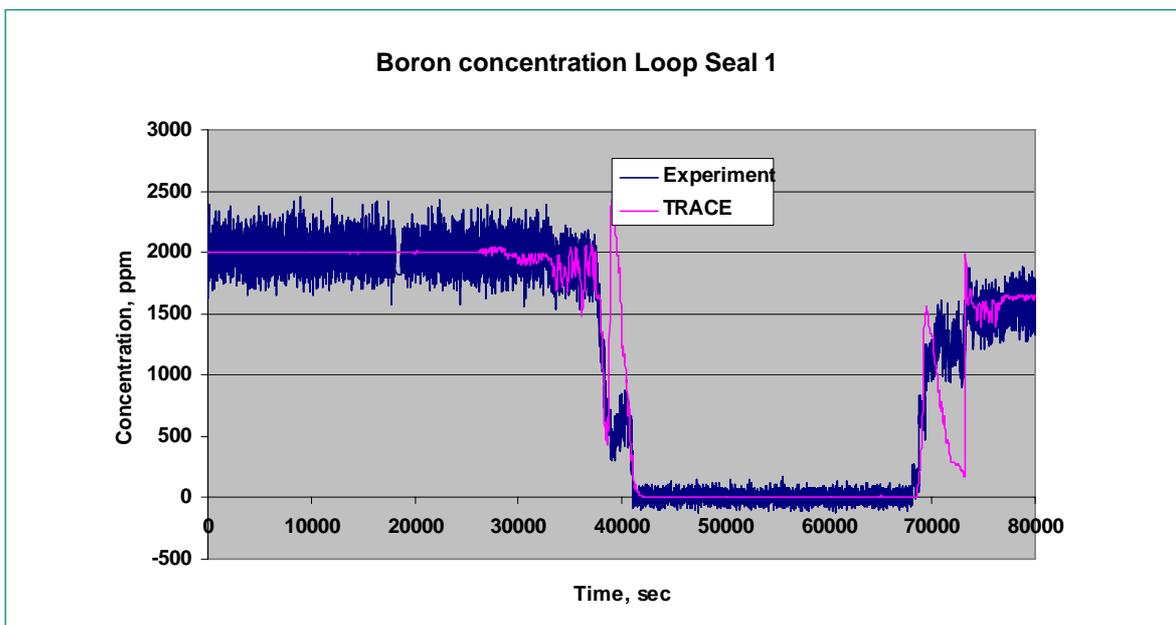
Figure 10: Boron concentration in a loop seal during PKL Test F1.2.
