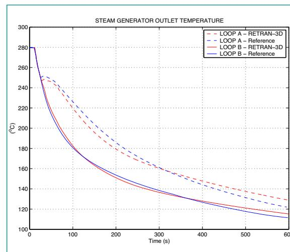
Figure 16: Comparison between the reference and the RETRAN-3D simulation of the steam generator outlet temperatures.
