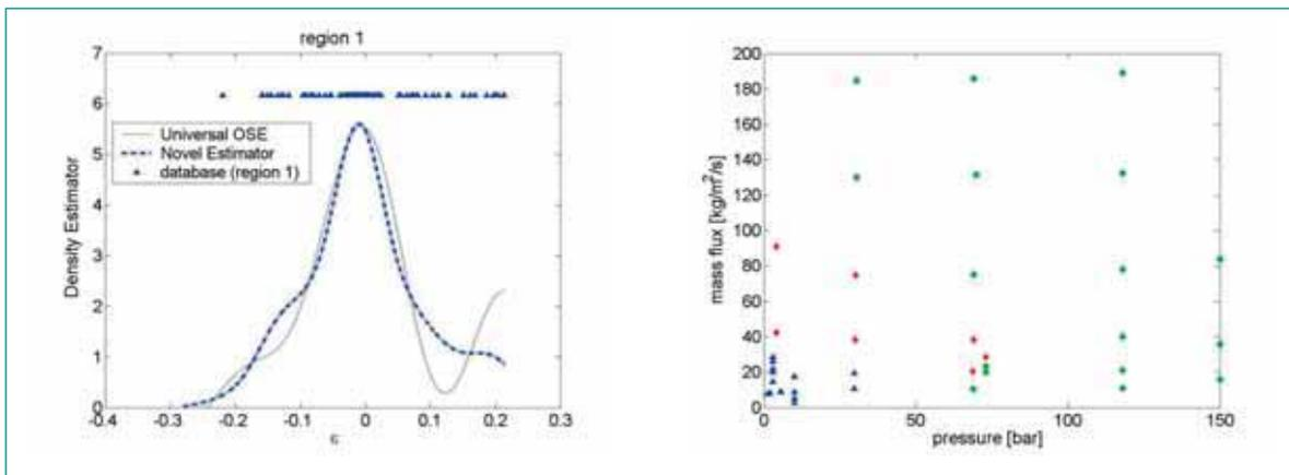
Figure 1: Pdfs base on the non-parametric estimator for void fraction uncertainty (*left*); two-dimensional clustering of the void uncertainty information (*right*) (each point represents a set of experimental values).
