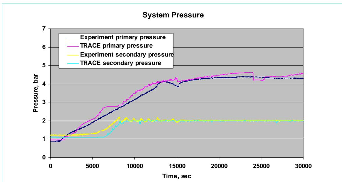
Figure 9: Primary and secondary pressure during PKL test E3.1.
