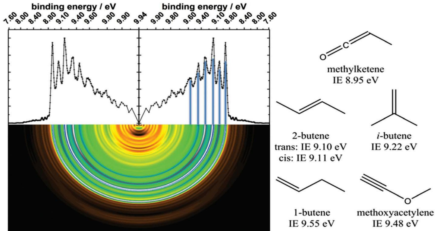
Photoelectron spectrum at  $h\nu = 9.94$  eV collected in coincidence with ions of mass 56 recorded from a methyl propionate / oxygen flame at a fixed height above the flame burner. The upper 2-D spectrum is the reconstructed PES of the lower image using the *p*Basex inversion procedure. Isomers of mass 56 that can contribute to the total signal are shown.
