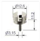
Special sample pin with 0.3mm diameter For very small samples
