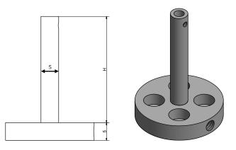
This sample holder is for pin diameter of 3.15mm
