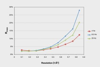
Speed comparison using lysozyme crystals and a PILATUS 6M-F. 180-degree datasets were collected at 4 Hz, 8.3 Hz and 25 Hz framing rate at constant angular speed. Datasets are of high quality at all framing rates (data courtesy of Dr. V. Olieric, PX beamline X06SA, PSI, Villigen, Switzerland).
