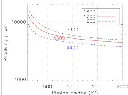
Calculated maximum resolving power (from ray tracing) for optimum source size 7 μm x 45 μm, horizontal acceptance 1 mrad, including optical aberration and nominal slope errors. Values at 1000 eV are indicated.
