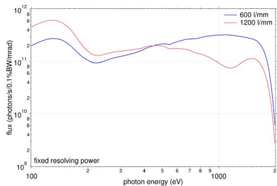
Calculated photon flux based on the dipole radiation spectrum and the transmission factors of the optical elements. The horizontal acceptance is 1 mrad, and the vertical acceptance infinite. The spectrum is normalized to constant resolving power 1000 and to 400 mA ring current.
