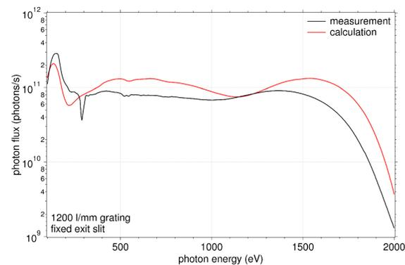
Maximum photon flux measured with a silicon photodiode. The calculated spectrum is normalized to the same acceptance (0.7 mrad H x 1.4 mrad V) and fixed exit slit size (200 μm). 200 μm correspond to a resolving power of about 1000 at 1000 eV. Currently, only a preliminary 1200 lines/mm grating has been commissioned.
