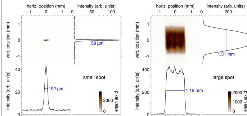
Beam spots at the sample position produced by the two toroidal refocusing mirror surfaces. The images are measured with a scintillator plate and a CCD camera. Profiles are integrated in the respective normal direction.
