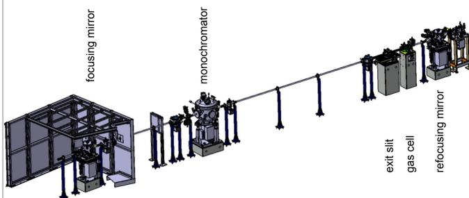
3D rendering of the beamline from focusing mirror unit to refocusing mirror unit.
