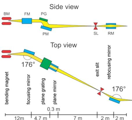
Plane-grating monochromator scheme operating in converging beam and negative diffraction order [1,4]. The X-rays are focused onto the exit slit by the focusing mirror and the plane grating. Drawing not to scale.
