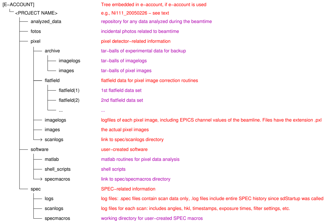
Figure 2.1: The structure of the directory tree created by sdStartup . Those branches whose comments are written in magenta are empty and have to be filled manually by the user. Those in red are filled automatically by SPEC during the experiment.
