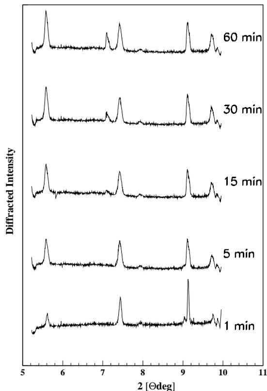
Fig. 5. Time development of the cement hardening process as recorded by the single module strip detector. The 1280 channels cover an angular range of about  $5^\circ$ .
