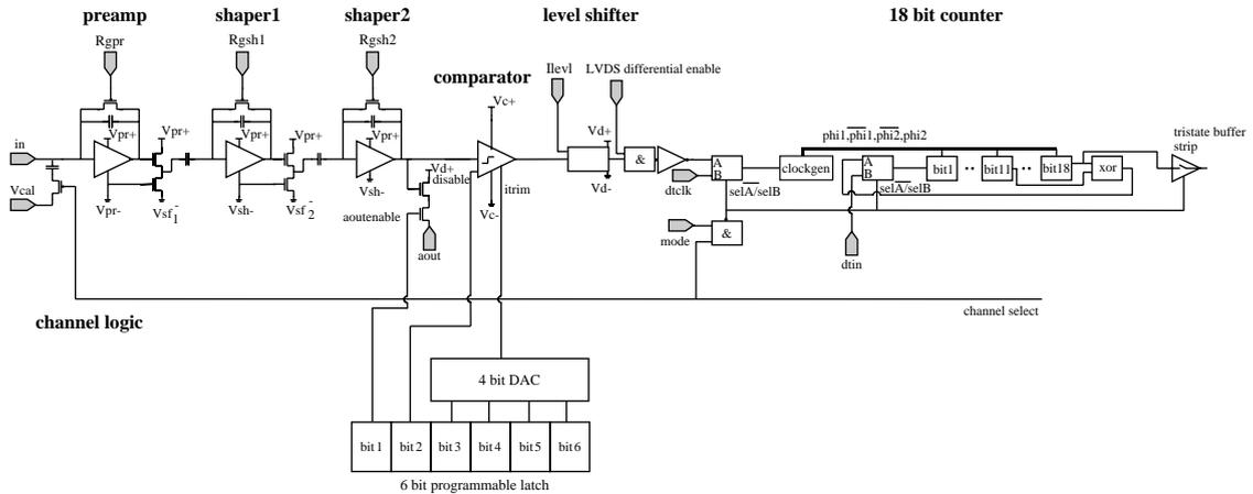
Fig. 3. Readout chip schematic. The chip consists of a global chip control logic (bottom part) and the channel electronics (upper part) which is identical for each of the 128 channels.
