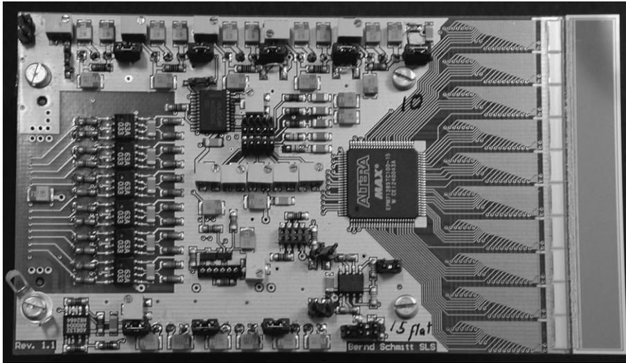
Fig. 2. The module control board. On the right side is the silicon sensor connected to the 10 readout chips by wire bonds. The module also carries voltage regulators, a DAC to supply the required voltages and additional electronics for chip selection. The size of the module is about  $11 \text{ cm} \times 6.5 \text{ cm}$ .
