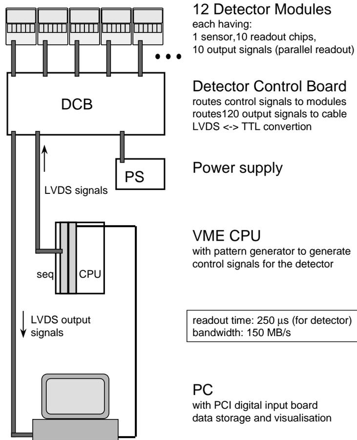
Fig. 4. Readout system. The complete detector system has been optimized for fast readout.
