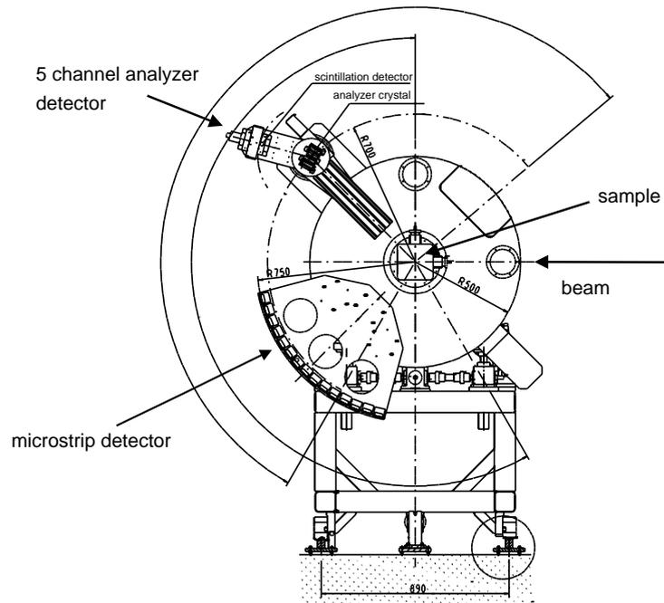
Fig. 1. Powder diffraction station at the material science beamline of the SLS. The sample is mounted in a capillary at the center. The five channel analyzer detector is used in the upper half of the diagram and the microstrip detector in the lower. Both systems can be used in parallel. The strip detector is mounted at a distance of 76 cm from the sample position.
