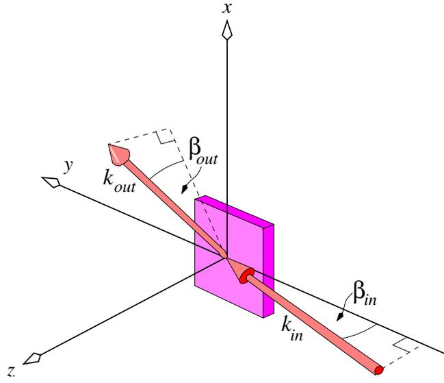
FIG. 3: Schematic of the incident and exit angles  $\beta_{in}$  and  $\beta_{out}$ . In the vertical geometry,  $\beta_{in}$  is equal to  $\alpha$ . In the horizontal geometry,  $\beta_{in}$  is equal to  $\omega_h$ .
