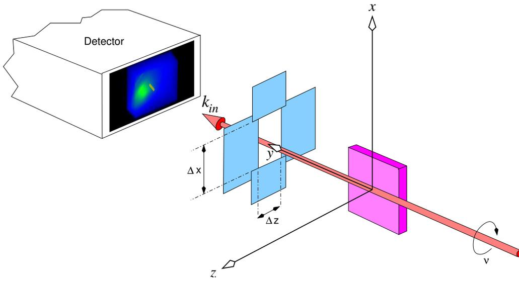
FIG. 4: Schematic figure of the detector and slit system for  $v = \alpha = \gamma = \delta = 0$ . The slit openings are  $\Delta x$  and  $\Delta z$ .
