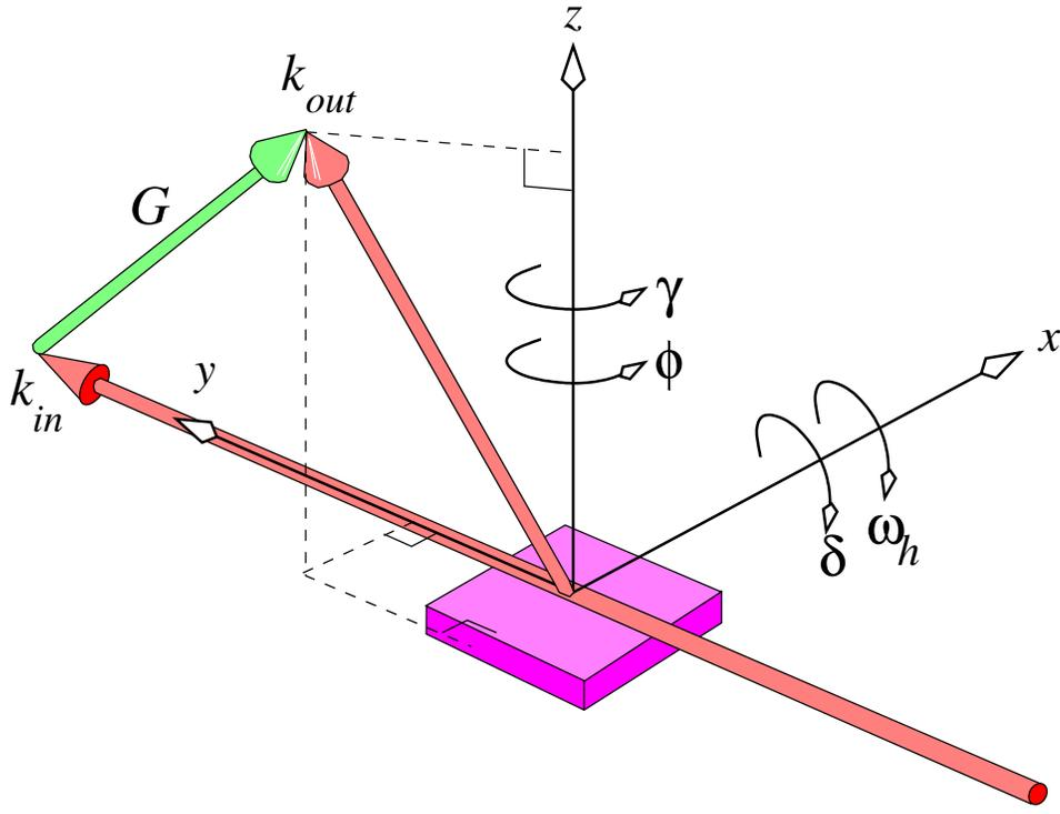
FIG. 7: Schematic figure of the laboratory coordinate system, incoming and outgoing wavevectors  $\vec{k}_{in}$  and  $\vec{k}_{out}$ , the scattering vector  $\vec{G}$ , and the pertinent motor rotations in the horizontal geometry setup of the surface diffractometer.
