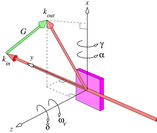
FIG. 2: Schematic figure of the laboratory coordinate system, incoming and outgoing wavevectors  $\vec{k}_{in}$  and  $\vec{k}_{out}$ , the scattering vector  $\vec{G}$ , and the pertinent motor rotations in the vertical geometry setup of the surface diffractometer.
