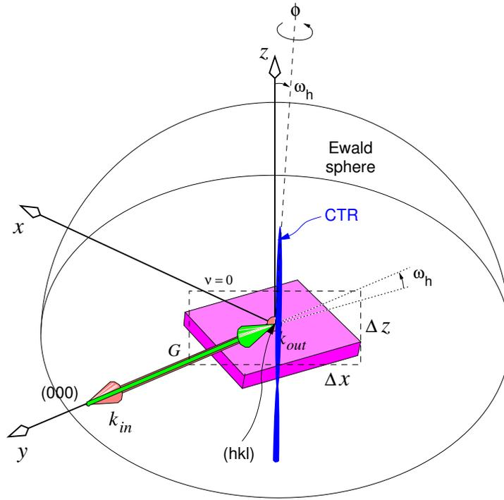
FIG. 8: Schematic figure of the vectors  $\vec{k}_{in}$ ,  $\vec{k}_{out}$ , and  $\vec{G}$ , as viewed from the perspective of the detector, which points back along  $\vec{k}_{out}$  towards the centre of the diffractometer (hence  $\vec{k}_{out}$  is seen here as being “head on”). The vector  $\vec{G}$  connects  $\vec{k}_{in}$  [at (000)] to  $\vec{k}_{out}$  [at (hkl)].
