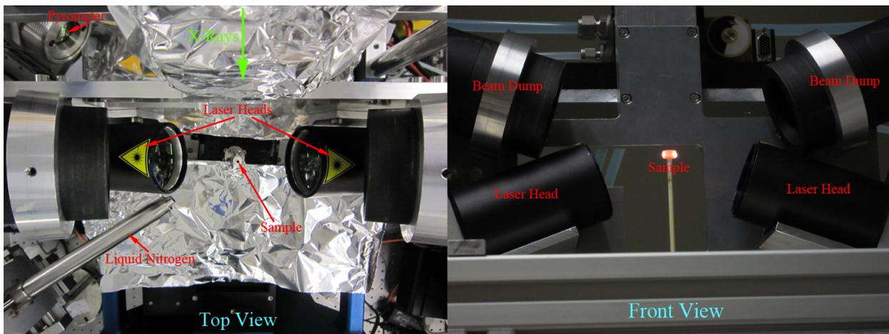
Figure 1. (L-R): Top and front views of the laser system on the TOMCAT beamline and in the lab respectively. The top view shows a sample holder 2mm in diameter at room temperature. The front view shows a sample holder 8mm in diameter being lased to approximately 1100°C.
