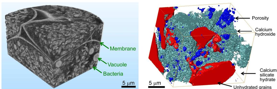
Phase tomography reconstructions. (Left) Bacteria inoculated cellular tissue from root nodules of the mung bean plant *Vigna radiata*. (Right) Hardened cement paste, segmentation was performed based on electron density.
