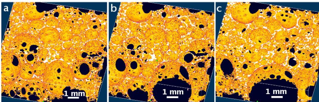
Figure 2 – The 3D dynamics of a rapidly evolving beer foam at three time instances (a:  $t_0$ , b:  $t_0 + 3$  sec, c:  $t_0 + 7$  sec) during natural coarsening. Total scan time was 0.5 s at 20 keV photon energy.
