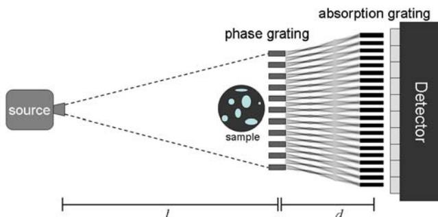
*Figure: Compact DPC setup consisting of a microfocus X-ray tube, a Talbot interferometer and a camera.*
