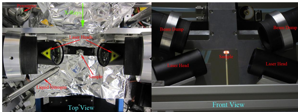
Figure 1. (L-R): Top and front views of the laser system on the TOMCAT beamline and in the lab respectively. The top view shows a sample holder 2mm in diameter at room temperature. The front view shows a sample holder 8mm in diameter being lased to approximately 1100°C.
