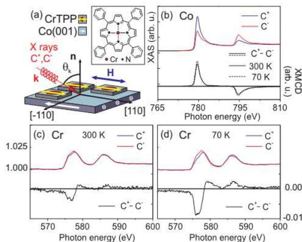
Figure 1. a) Sketch of the experimental setup. b) XMCD signal of the ferromagnetic cobalt substrate measured at Co  $L_{3,2}$  edge c),d) XMCD spectra of Cr  $L_{3,2}$  edge reveal and antiferromagnetic coupling of CrTPP molecules with respect to substrate magnetization.
