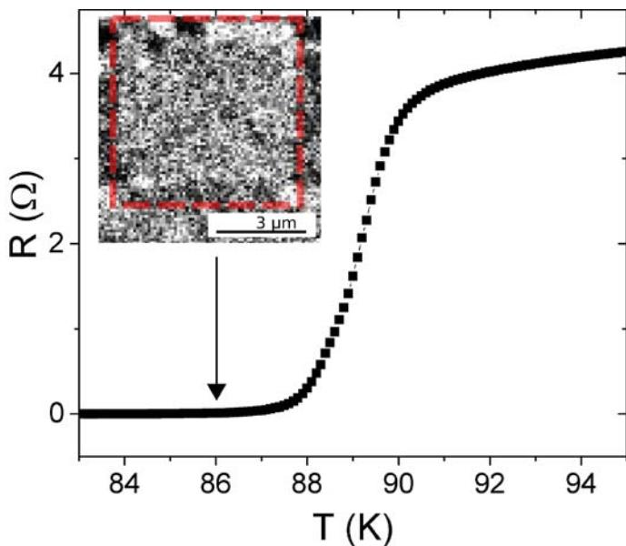
Figure 1: Resistance versus temperature curve of YBCO thin film indicating the  $T_c$  of 89 K. Inset: XMCD image of a 6  $\mu\text{m}$  Py square taken at 86 K. The square is highlighted with red dashed line, dark cross corresponds to the out-of-plane magnetization component.
