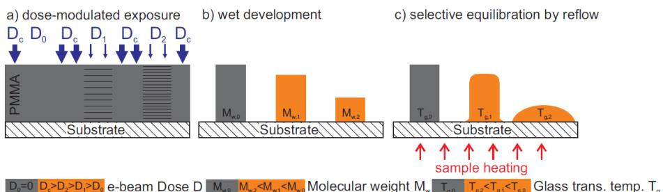
**Fig. 1:** Schematic of the process flow combining electron beam grayscale lithography and polymer reflow for selective pattern equilibration.
