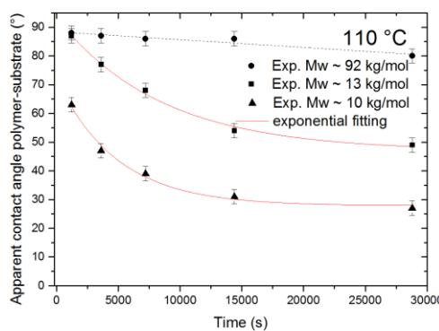
**Fig. 2:** Evolution of the apparent contact angle
