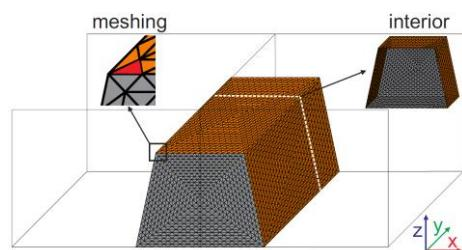
**Fig. 3:** Initial geometry for a reflow simulation of a single line demonstrating the triangular meshing and the soapfilm-approach.
