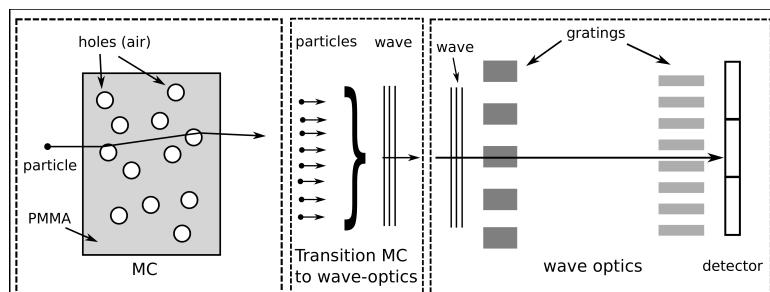
Figure 1: Sketch of the simulation framework
