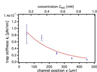
Figure 3. Trap stiffness of 60 nm gold particles recorded at different positions in the nano-channel. The higher the ionic strength of the solution, the less strong the particles are confined in the traps.
