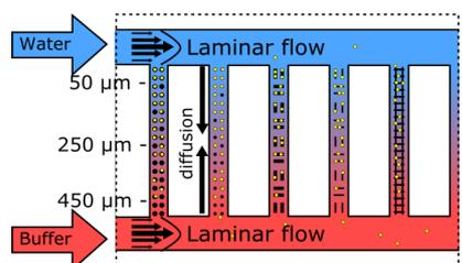
Figure 2. A steady state gradient in the trapping region is formed by simple diffusion of the salt ions from the two buffer solutions flowing through the supporting channels. Thus the analysis of single nano-objects at different concentrations is achieved within a single device.
