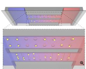
Figure 1. Schematic of nano-objects trapped along a steady linear reactant gradient by combining GIE trapping devices with a microfluidic design.
