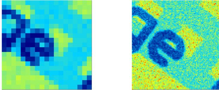
Figure 1: Examples of MÖNCH position resolution. Left: absorption image of an HDI, in photon counts per pixel. Right: same image, after position interpolation, with 1  $\mu\text{m}$  bins.
