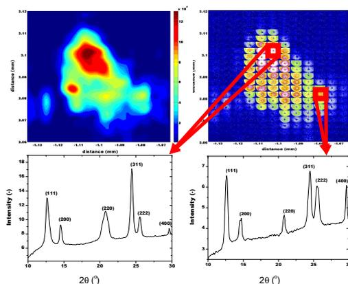
Figure 1: Examples of micro-XRF and micro-XRD maps of the irradiated fuel particle, and integrated diffraction intensity plots from two different regions in the fuel particle are shown.
