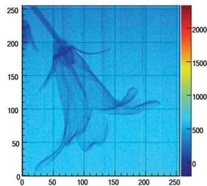
Figure 1: First JUNGFRAU 1.0 prototype module (left), X-ray transmission image of a flower recorded with JUNGFRAU 1.0 (right).
