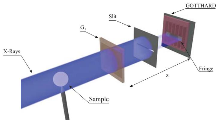
Fig. 1 Setup of the G2-less grating interferometer. The microstrip detector is placed at a distance of  $z_1 = 15$  cm downstream of the G1. The microstrips have a length of several mm and therefore the beam is additionally collimated by a  $2\mu\text{m}$  tungsten slit directly in front of the sensor.
