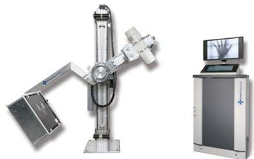
Demonstrator system. Our detector is on the bottom left.
