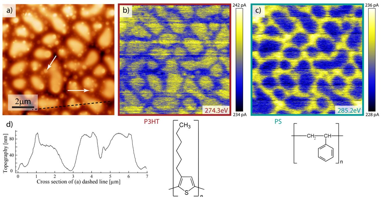
**Fig. 1:** Successive measurements performed on a P3HT/PS polymer blend. (a) AFM shows the topography of the sample. (b, c) STXM images recorded in situ at the same sample position at two different energies highlight the P3HT and the PS rich phase.
