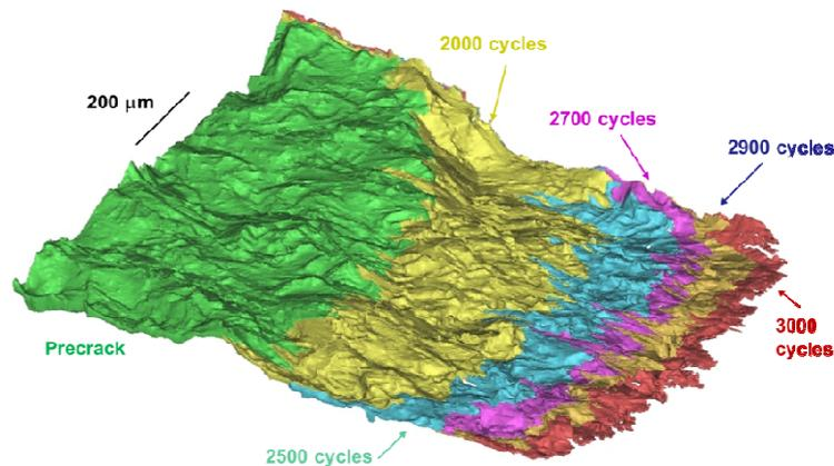
Figure 1. 3D reconstruction of fatigue cracking in 7075 Al alloy as a function of cycles.
