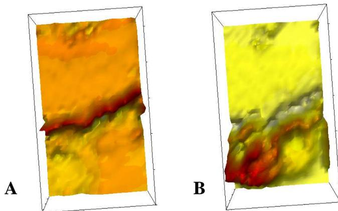
**Figure 1.** Distribution of inorganic salts in a weathered paint chip based on contrast generated by mid infrared absorption from oxoanions. Red corresponds to high absorption and white to no absorption. A – Carbonate. B – Oxalate.
