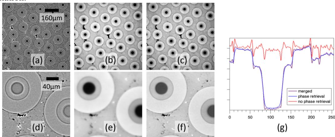
**Fig 1:** SiC fiber composite sample by a) standard slice reconstruction b) slice after phase retrieval of projections, c) slice containing merged information from slices a) and b). Corresponding zoomed-in regions are shown in d), e), and f). A line profile is shown in (g) for direct comparison.
