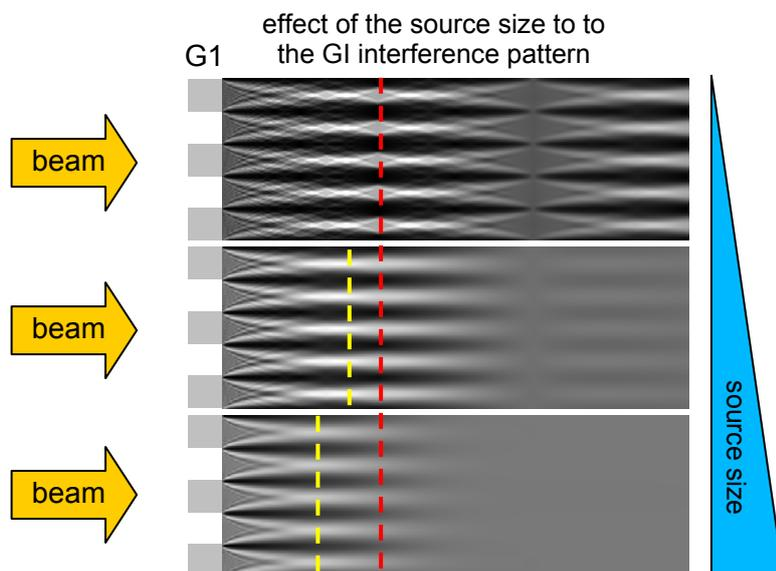
*Fig. 1: Interference patterns generated by a phase grating (G1) for different focal spot sizes of the source (source size). A sample is typically placed directly upstream of G1. G1 shifts the phase of the wave front periodically by  $\pi$ . An increasing source size attenuates the intensity of the interference fringes at larger distances, which reduces the detectability of sample refraction.*
