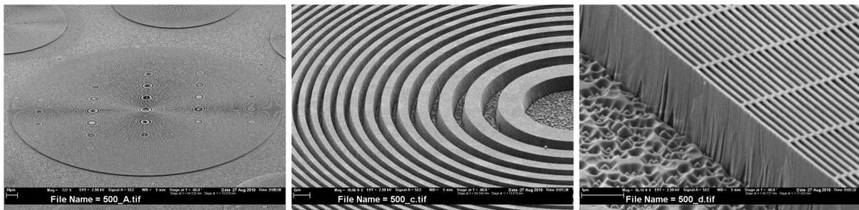
**Figure 1:** Scanning electron microscope image of a 500- $\mu\text{m}$  in diameter Fresnel zone plate capable of collecting a full coherent XFEL beam. The FZP has a 100 nm outermost zone and etched 2.2  $\mu\text{m}$  deep into a CVD diamond layer. (from left to right) Overview of the zone plate, central zones and outermost zones.
