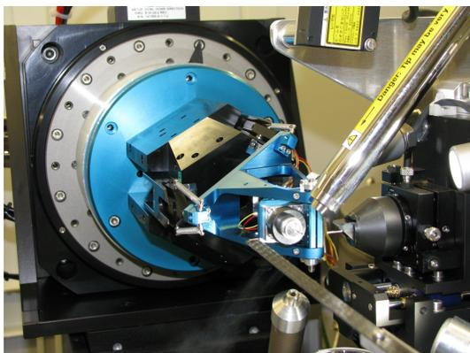
Figure 1: The multi-axes goniometer PRIGO installed at X06DA
