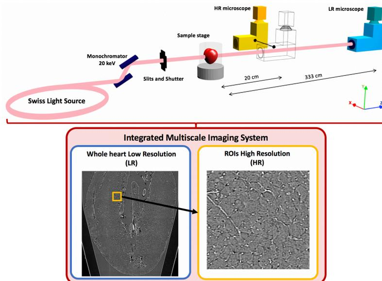
Figure 1. Sketch of the multiscale imaging setup at the TOMCAT beamline.
