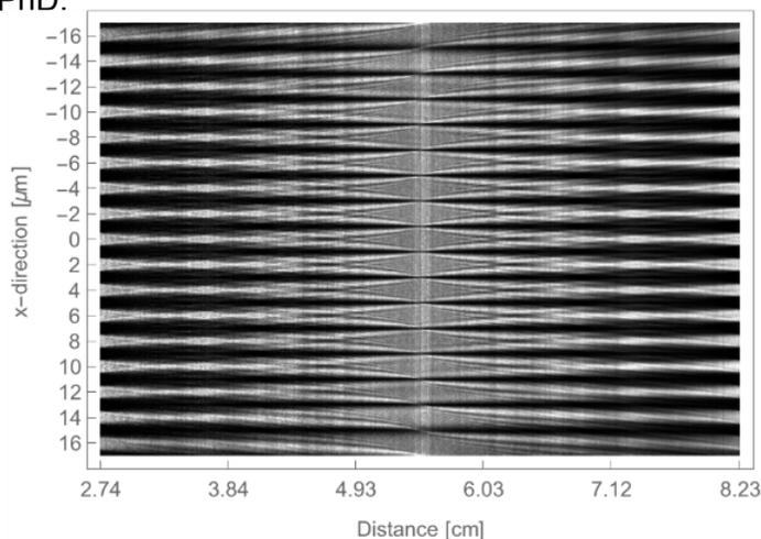
**Figure 1.** Talbot carpet simulated with a Huygens principle MC.
