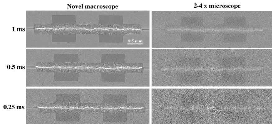
**Figure 1** Tomographic slices of a fuel cell sample. Left: reconstructions from novel macroscope images. Right: reconstructions from images acquired with the previously used high temporal resolution setup. For both imaging setups the projection exposure time was from top to bottom 1 ms, 0.5 ms and 0.25 ms. All reconstructions were created from evenly spaced 400 projection images acquired using monochromatic beam energy of 13.5 keV.
