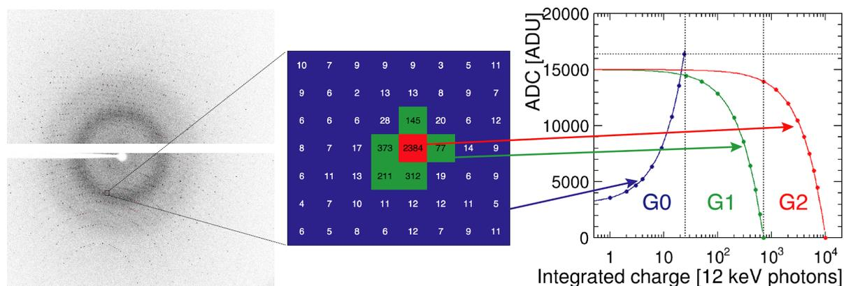
**Figure 1** A diffraction pattern measured with a JUNGFRAU 1Mpixel detector and an illustration of the extended dynamic range with three gain levels (G0, G1 and G2).
