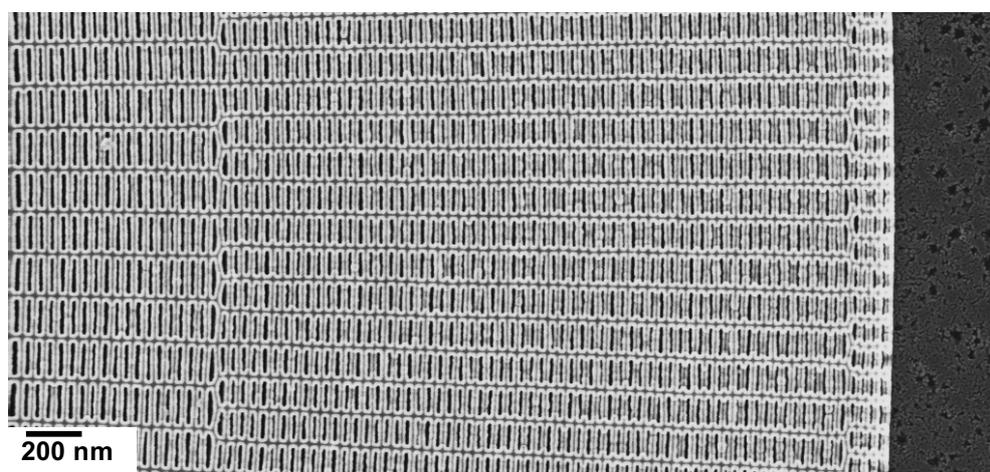
Figure 1: Fresnel zone plate with line-doubled iridium zones of 9 nm line width.
