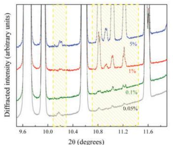
SR-XRPD patterns recorded on pharmaceutical binary mixtures of similar elemental composition ranging from 0.05% to 5% weight (wt) of the minority phase. The small XRPD signal is directly detectable down to 0.05% wt with a signal-to-noise better than 10, allowing the quantification of the minority phase
