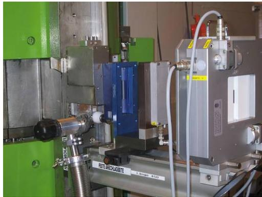
Neutron monitor and motorized slit after the monochromator.
