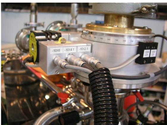
Motor Controller for Sample Rotation
