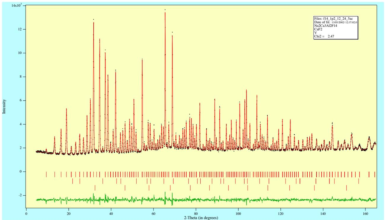
Fig. 12a: Observed, calculated and difference neutron diffraction pattern of  $\text{Na}_2\text{Ca}_3\text{Al}_{12}\text{F}_{14} + \text{CaF}_2 + \text{V}$  from the sample container (sample diameter 5 mm) with  $\delta 2\theta = 0.05^\circ$  for  $2\theta_M = 120^\circ$ ,  $\lambda = 1.197 \text{ \AA}$ ,  $\alpha_1 = 12'$  and  $\alpha_2 \approx 24'$ .
