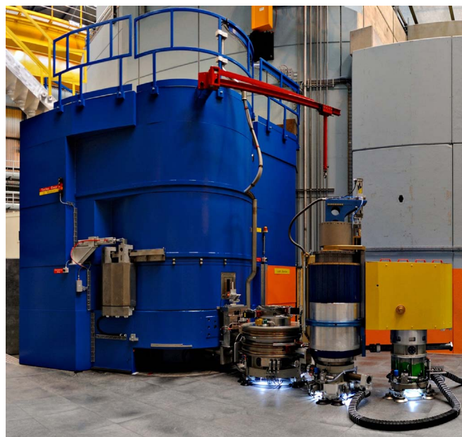
Fig. 3. Picture of the monochromator shielding, sample table and the secondary spectrometer with the analyzer housing and the detector shielding of EIGER.
