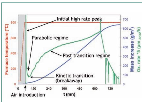
Figure 4: Illustration of results from MOZART tests on air oxidation of Zircaloy cladding at 800° C, showing transition to breakaway regime (Duriez, priv. comm., 2006)
