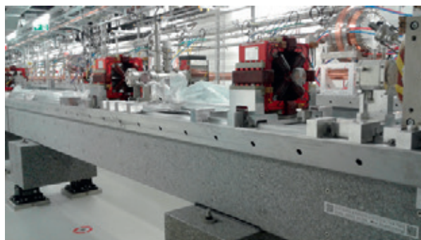
Fig. 3.8.1.1: Granite girder sitting on 4 feet. Each feet is manually adjustable in x, y and z. The components (e.g. quadrupoles) are positioned with shimming blocks on the precisely machined granite surface.
