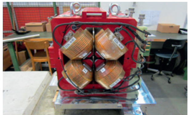
Fig. 3.4.1: QFF quadrupoles from SwissFEL (left picture) with integrated horizontal and vertical steering function. QFM quadrupole from SwissFEL water cooled (right picture).
