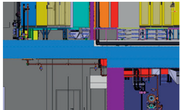
Fig. 5.1.5: Top view of the RF gallery the Athos C band module (top picture). The waveguide crosses the floor and goes through the UH.006 room and then into the tunnel (bottom picture).
