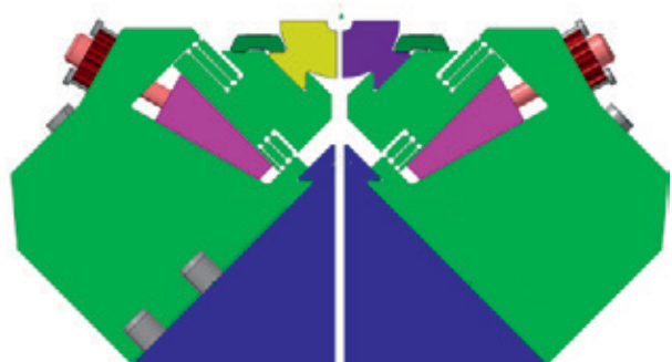
Fig. 3.5.8: Front view of the keepers holding the magnets at 45 degrees in the undulator Athos.
