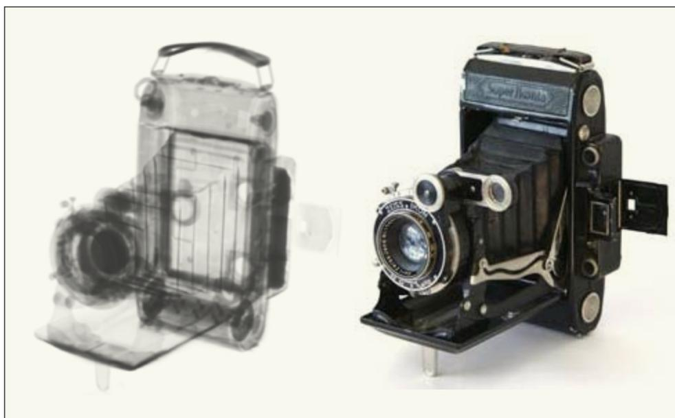
Photograph (right) and transparent neutron tomograph (left) of an old camera. With neutron tomography the inner structure of the camera is unveiled.
