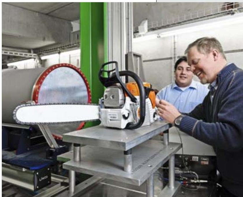
Setting up a real-time experiment (stroboscopic mode) with a combustion engine driving a chain saw (results below).
