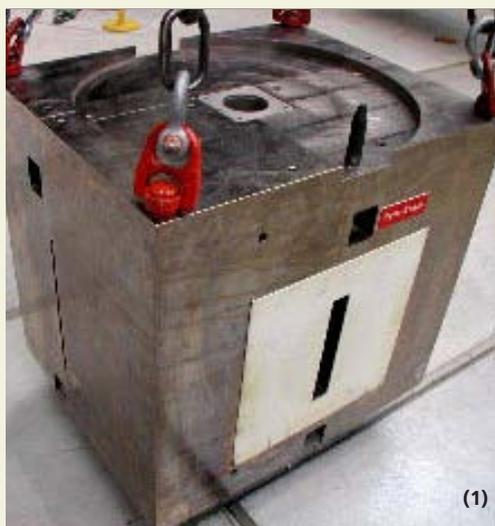
NEURAP setup with shielding block (1) and transport cask (2) containing the sample manipulator.
