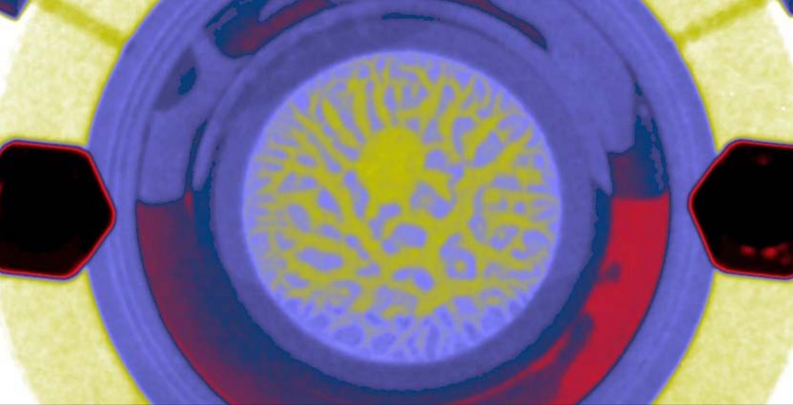
**Battery research: distribution of the electrolyte inside the battery, visualized with neutrons.**
