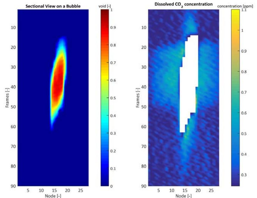
Sectional view on a CO<sub>2</sub> bubble in terms of void and dissolved CO<sub>2</sub>
