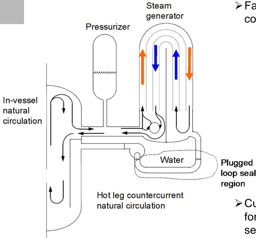
➤ Failure of SG tubes before Hot Leg → containment bypass scenario
