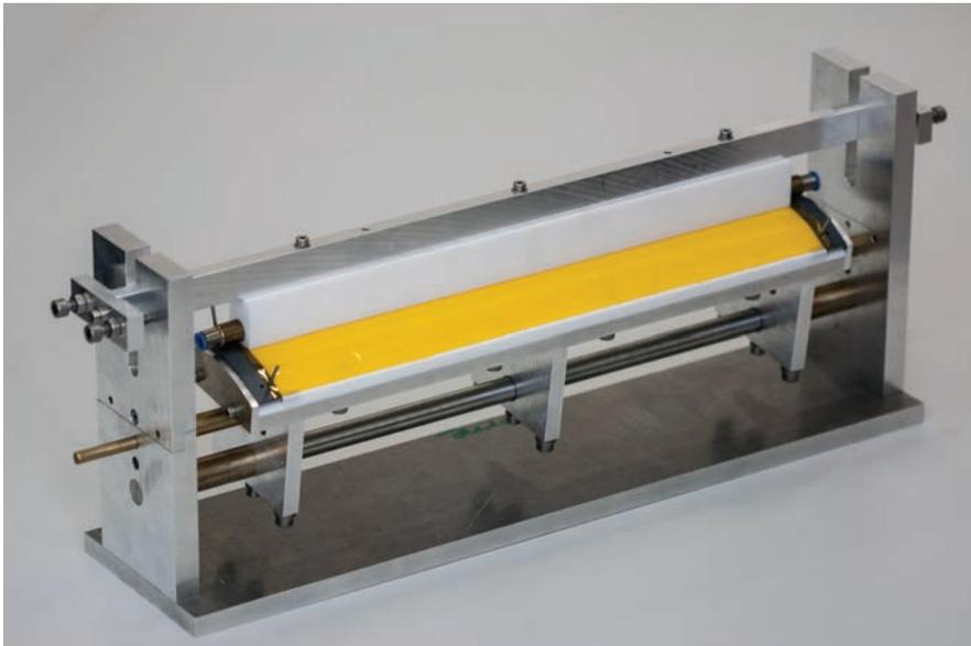
Figure 3.3: Assembly tool for outer layer modules
