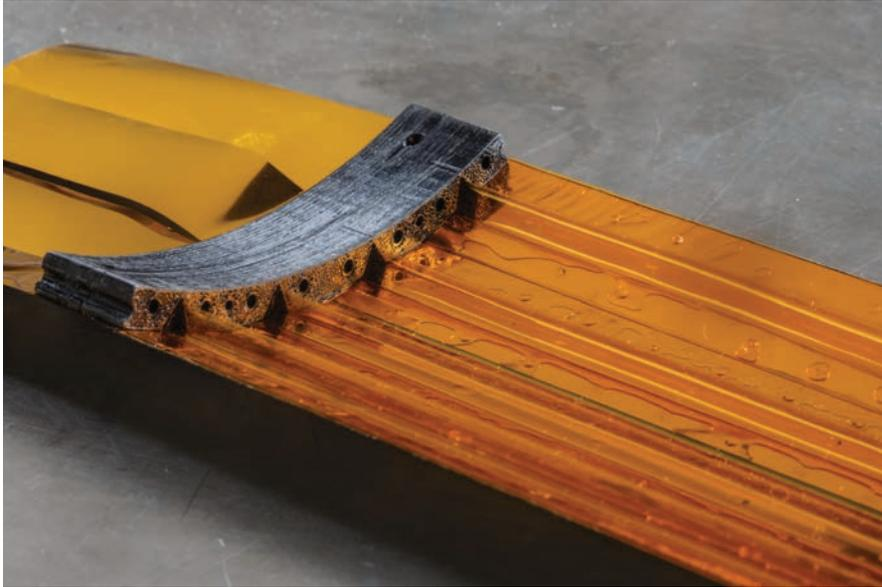
Figure 3.2: Kapton foil with supporting structure glued on an end-piece
