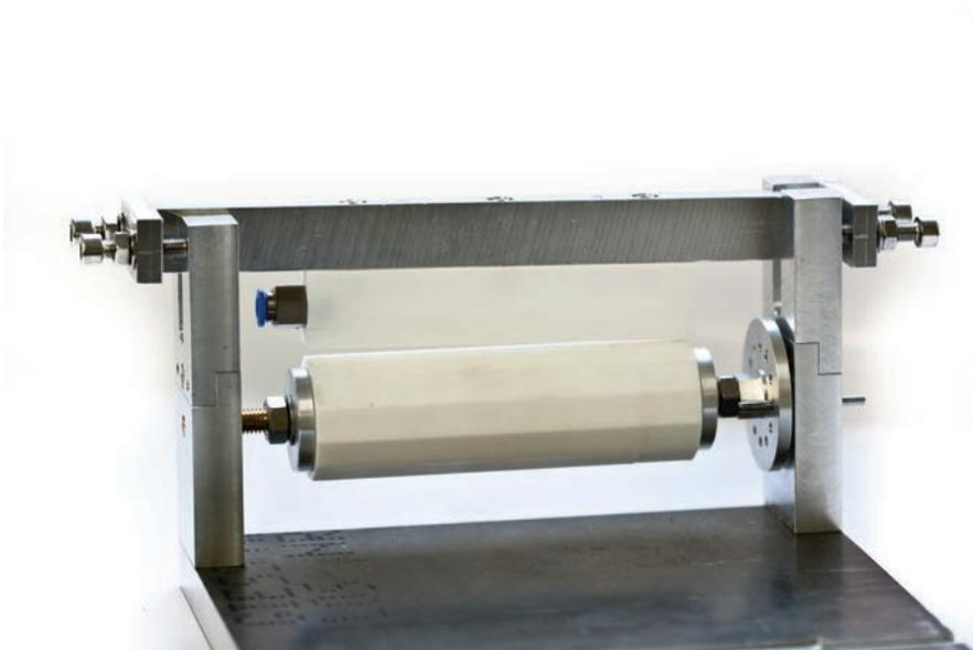
Figure 3.5: Assembly tool for the inner layer prototype
