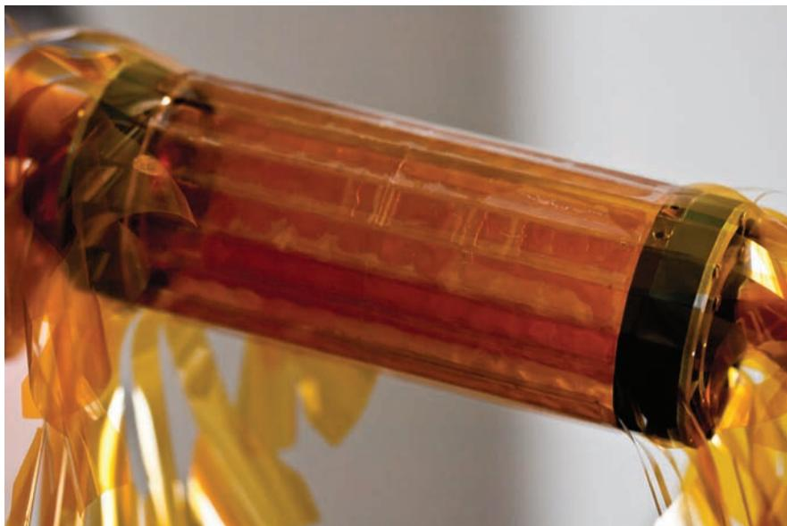
Figure 3.6: A mechanical prototype of the inner detector station, with sensor layer 1 and 2
