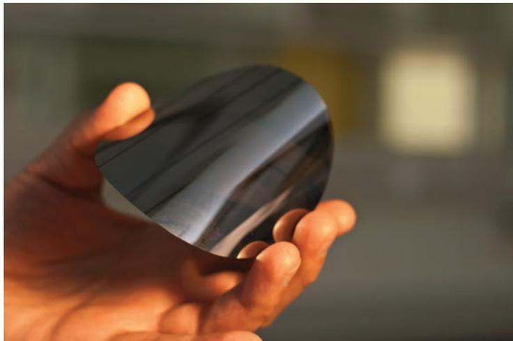
Figure 2.13: A  $50\mu\text{m}$  thin silicon wafer
