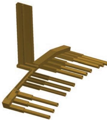
Figure 5.8: CAD model the Gas inlet for the simulation
