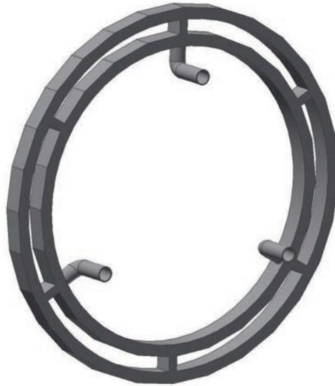
Figure 7.1: The CAD model (with 3 gaseous inlet) for an compact end-ring
