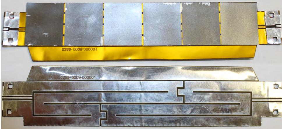
Figure 5.4: Up- and downside of one tape heater with steel plate on top and aluminium resistor on downside.
