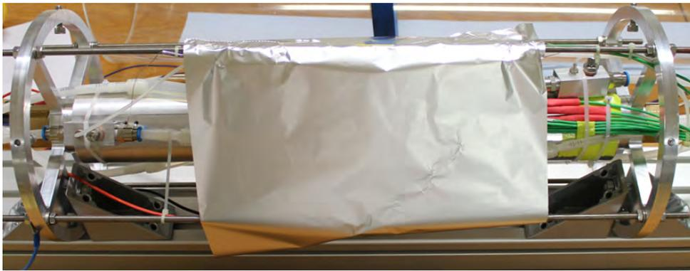
Figure 5.26: Aluminium shield over the mockup to investigate the heat radiation.
