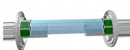
(c) The scintillating fiber ribbons of the timing tracker.
