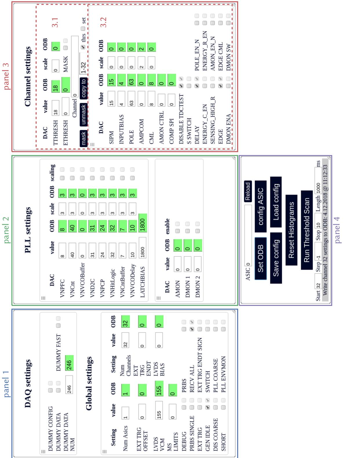
Figure C.3: MIDAS based MuTRIG Configuration GUI. Standard settings for operation for the scintillating fibre detector are shown.
