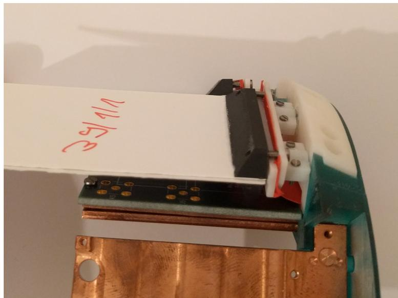
**Figure D.2:** 3d-printed model of the mechanical integration of the scintillating fibre detector into the  $\mu$ 3E experiment.
