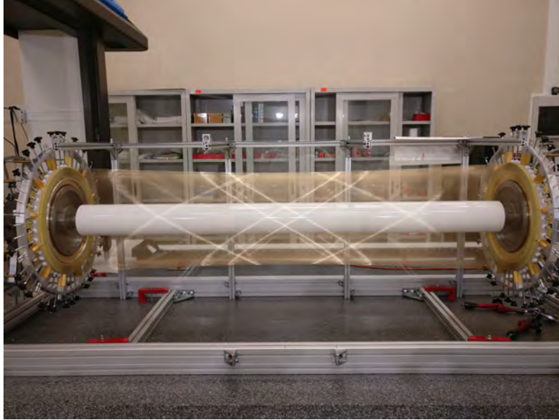
Figure 1.15.: [43] Shown is the production status of the MEG II CDC with approximately 50 % of the final \sim 1200 sense wires and \sim 6400 field wires being installed. The picture was provided by Marco Chiappini.
