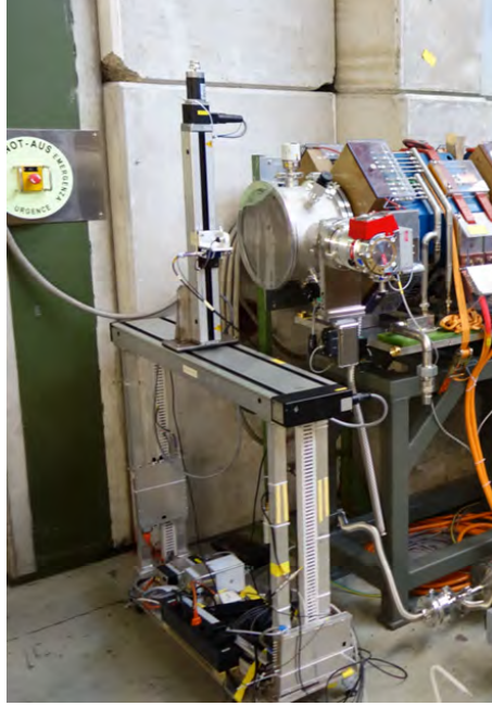
Figure 4.11.: Shown is the new XY-scanner that has been employed for all measurements in the front part of the \pi E5 area, that are presented in this thesis.
