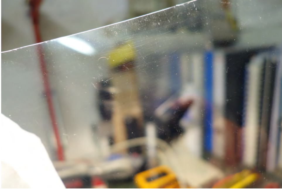
Figure 3.22.: The close-up image shows inhomogenities and scratches in the scintillator surface that can be identified in the beam picture 3.21.
