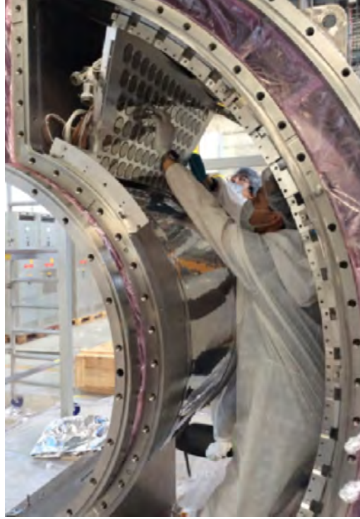
Figure 1.19.: [43] Shown is the replacement of the inner layer PMTs with dedicated SiPMs from Hamamatsu, which has already been finished.
