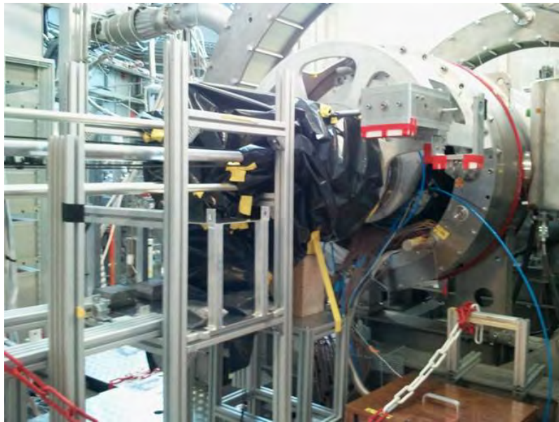
(b) Light-tight plastic foil covers the camera-mirror support
