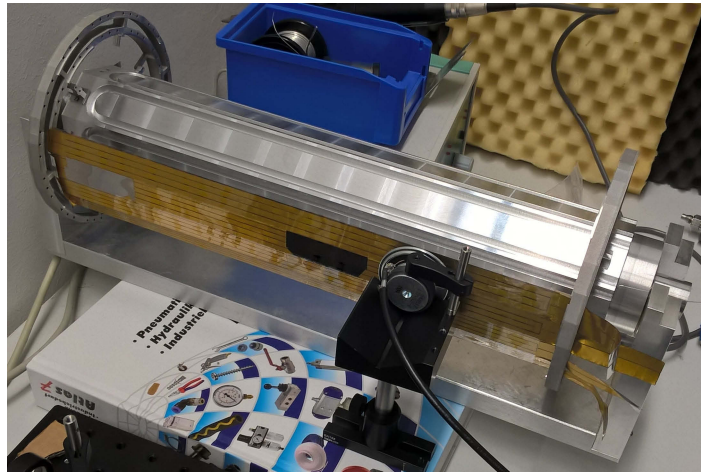
Figure 4.9: Layer 3 module prototype with beam pipe prototype. The speaker in front of the module was used for frequency response measurements (chapter 5) and is not part of the module mounting.
