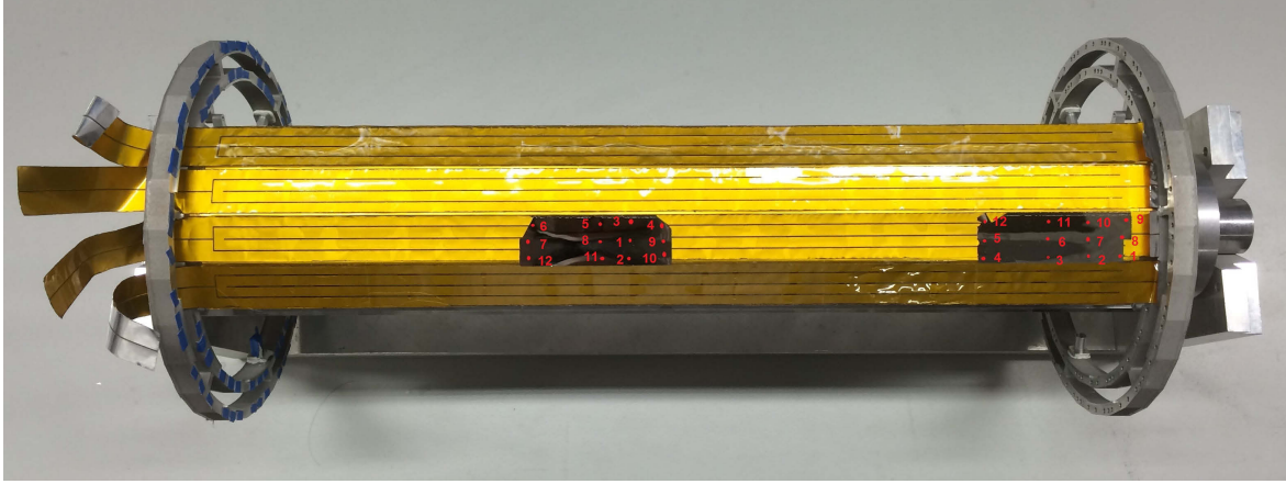
Figure 8.1: Laser reflection points in the deformation measurement of the layer 3 module
