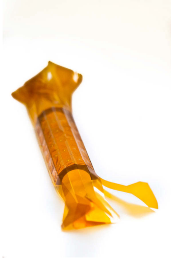
Figure 3.16: Mechanical prototype of an inner layer module
