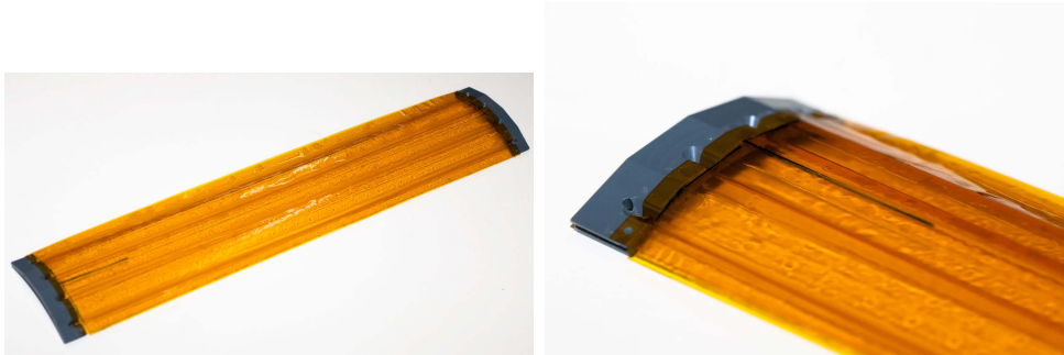
Figure 3.17: Mechanical prototype of an outer layer module
