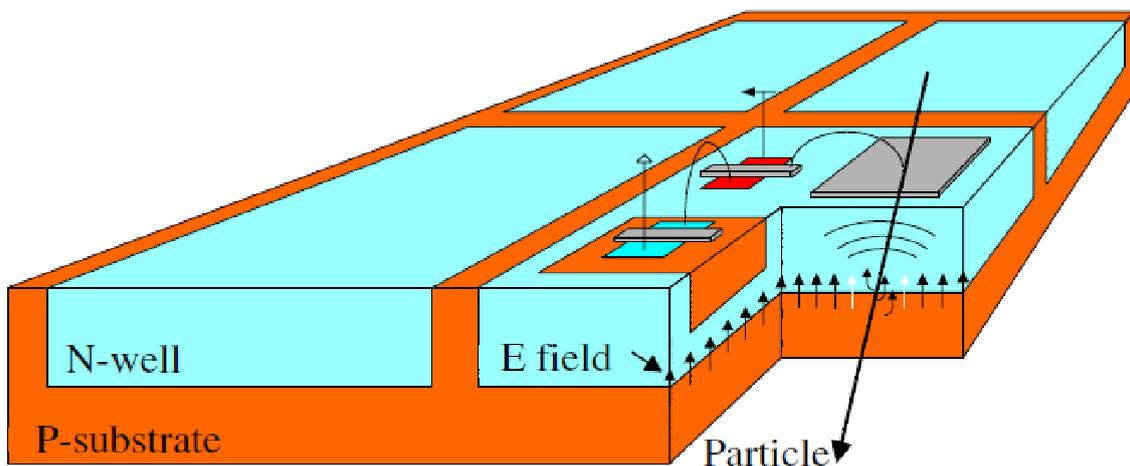
Figure 6.1: Simplified HV-MAPS pixel concept [21]
