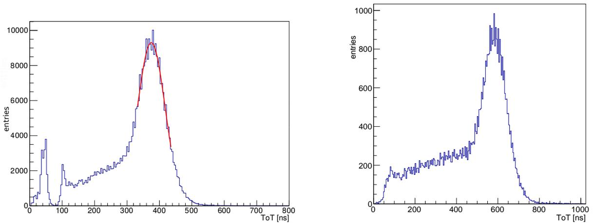
(a) ToT histogram of a single staged MuPix6 pixel with the iron source
