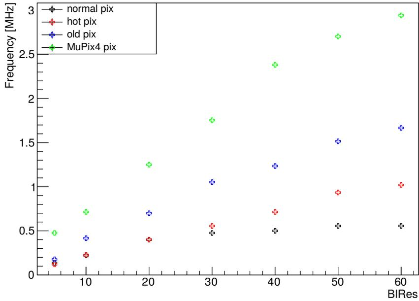
Figure 10.15: Plot of the BIRes dependence of the oscillation. The period was measured and the frequency calculated from the period. The values are not representative as the noise introduces variations in the period for multiple measurements and only one pixel was measured for each type. "old pix" refers to an one staged pixel on a MuPix6 chip.
