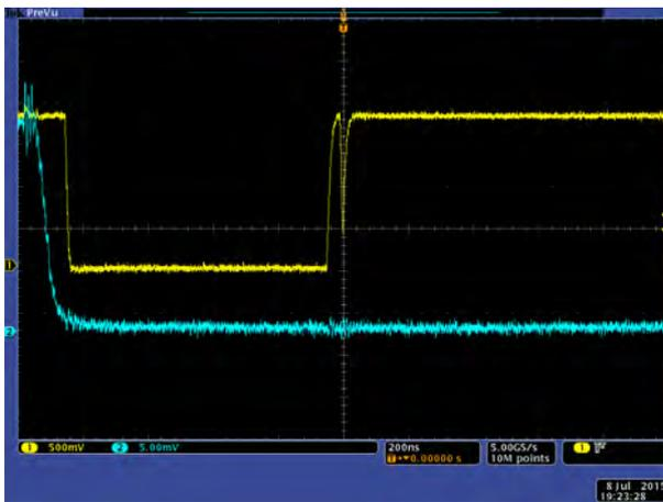
(a) Comparator pulse with one afterpulse (yellow) and the triggering injection (teal)
