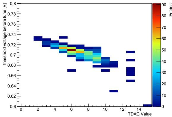
(a) 0.1Hz noise rate threshold before tuning vs TDAC value
