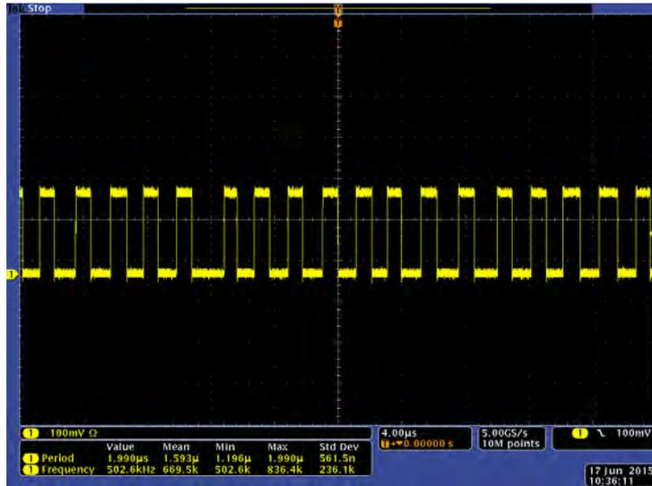
Figure 10.14: Comparator oscillation in a MuPix4 pixel
