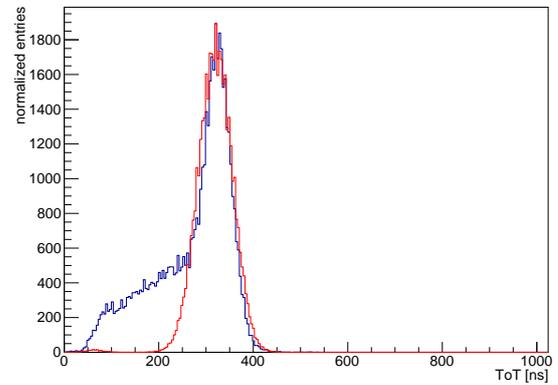
(b) ToT histogram of a MuPix4 pixel with the iron source (blue) and the injection (red).
