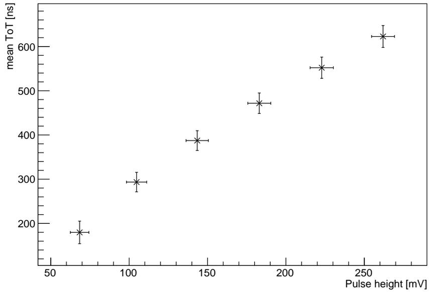
Figure 10.35: Pulseheight vs ToT for a MuPix6 pixel with one amplification stage
