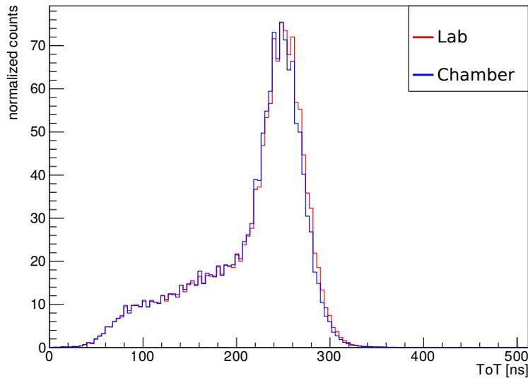
Figure 10.4: ToT histogram of the Fe55 source with (blue) and without (red) the climate chamber. The histograms have been normalized to match each others integral
