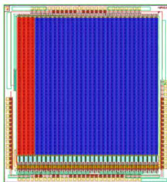
Figure 7.2: The MuPix6 Chip Layout exported from Cadence<sup>®</sup> Red: 1-staged pixel, blue: 2-staged pixel.
