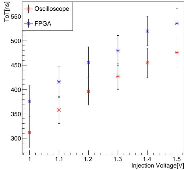
Figure 9.1: ToT measured with an oscilloscope and the FPGA for different injection voltages
