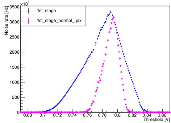
(a) Noise rate depending on stages switched on. The names in the legend refer to the stage that was last switched on. This means that the mentioned stage and every stage afterwards is turned on while every stage before is turned off
