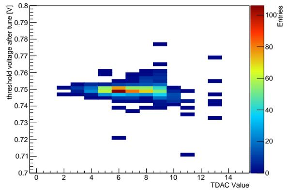
(b) 0.1Hz noise rate threshold after tuning vs TDAC value
