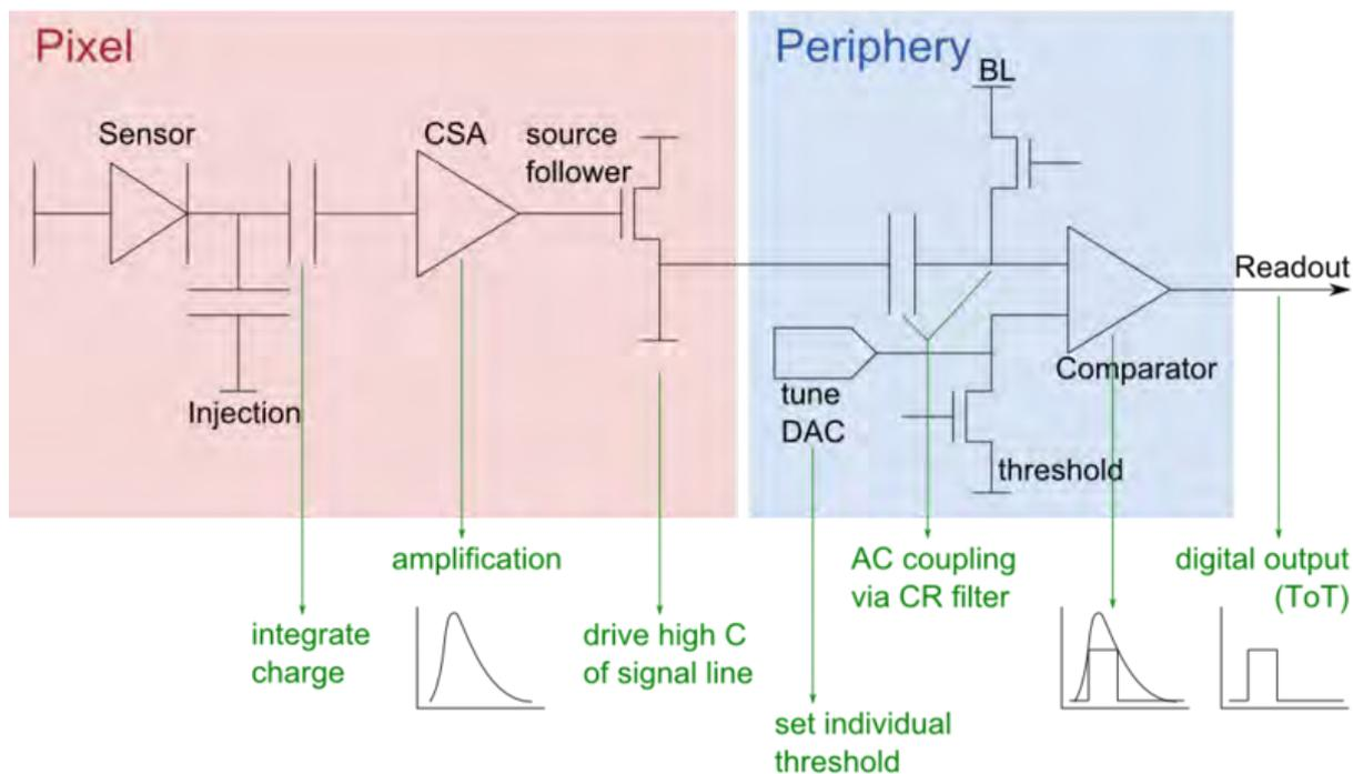
Figure 7.7: Drawing of the pixel and periphery of a MuPix4 and their effect on the pulse.
