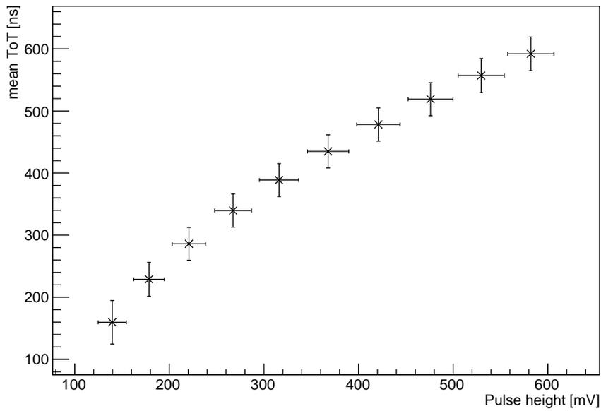
Figure 10.34: Pulseheight vs ToT for the MuPix6. Each point is for a different injection voltage (Fig. 10.32).
