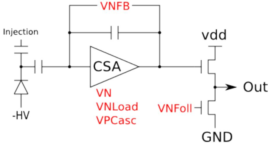
(a) Simplified schematic of the in-pixel logic. "Out" is the line to the periphery.
