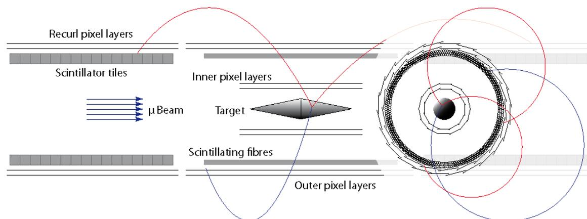
Figure 3.4: Design of the Mu3e detector with a  $\mu \rightarrow eee$  decay. The view on the right side is along the beam axis.
