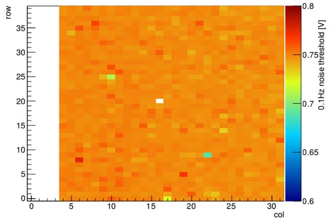
(b) 0.1Hz noise threshold pixel matrix after tuning
