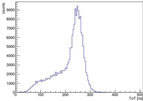
(a) ToT histogram of a MuPix4 pixel with the iron source
