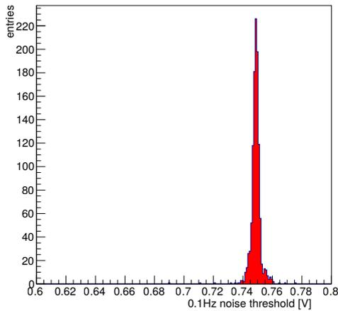
(a) 0.1Hz noise threshold distribution after tuning
