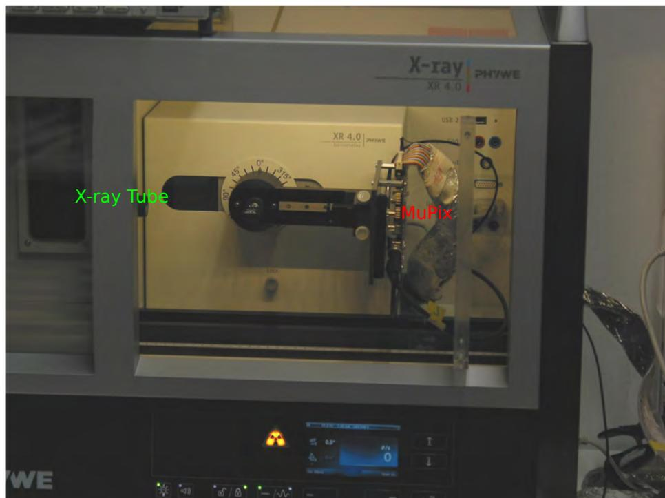
Figure 8.5: The MuPix placed in the X-ray spectroscope [36]
