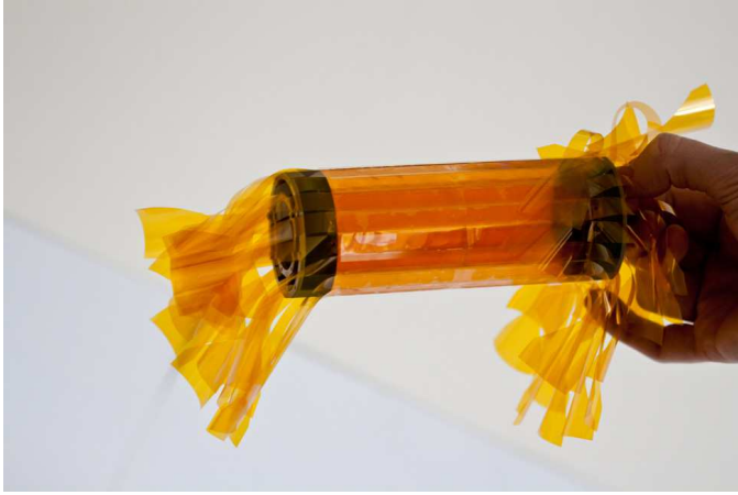
Figure 5: Prototype of the inner layer mechanical structure. The sensor chips are simulated by 100\mu\text{m} thin glass plates.
