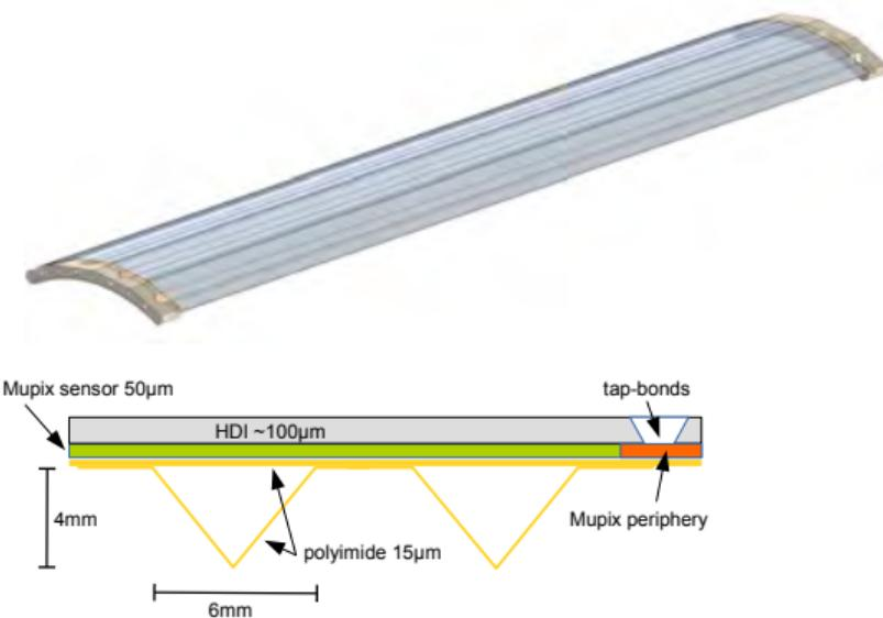
V-shaped groove for stability and cooling
